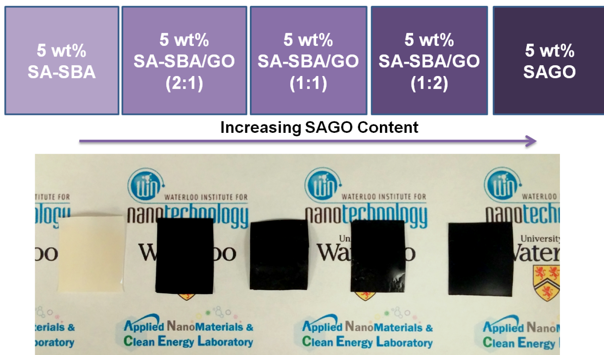
Figure 4.12: Physical membrane comparison with increasing SA-GO content versus SA-SBA
