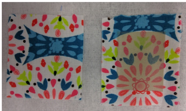
Figure 2.33: NW coating on cotton patterned fabric The left image shows the fabric without the NW coating and the right image shows the fabric after NW coating
