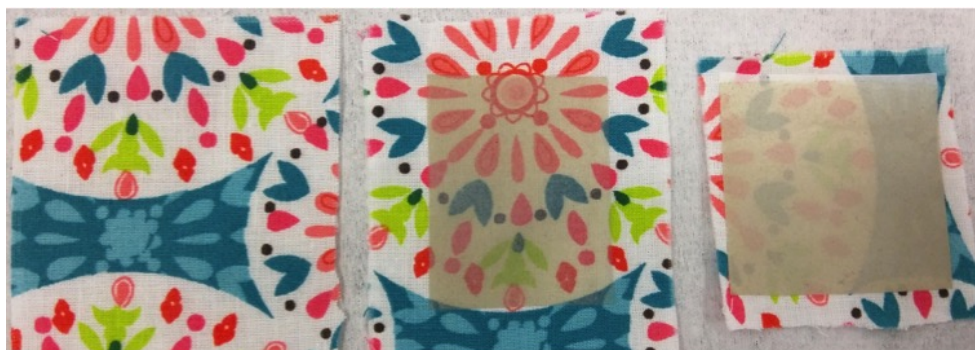
Figure 2.37: Transparency comparison between light and dark transfer paper. The first panel is a regular printed cotton cloth. The second panel is a printed cotton cloth coated with AgNW network using light transfer paper. The third panel is a printed cotton cloth coated with AgNW network using dark transfer paper.
