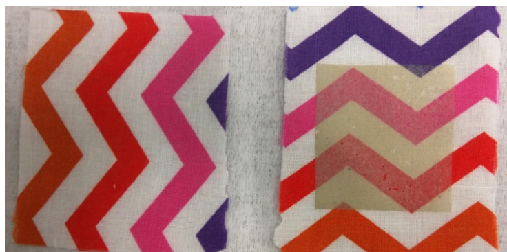
Figure 2.34: NW coating on cotton patterned fabric The left image shows the fabric without the NW coating and the right image shows the fabric after NW coating
