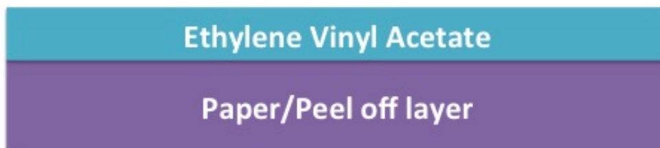
Figure 2.12: Schematic of light transfer paper
