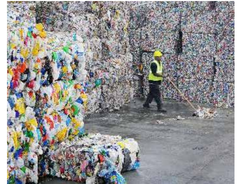
Figure 6.16: Recyclables after delivery, sorting being done manually, sorted and banded recyclables ready to be sent to a manufacturer.
