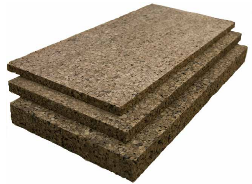
Figure 4.6: Expanded cork insulation. Cork comes largely from Portugal and is classified as a rapidly renewable material, but its limited supply will never be able to replace plastic insulations in the quantities we use today. However, it might be useful in specialized applications for its fire retardant qualities..
