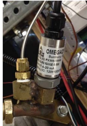
Figure 4.5 Thermocouple & pressure transducer
