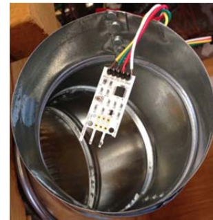
Figure 4.6 Air temperature & velocity sensors
