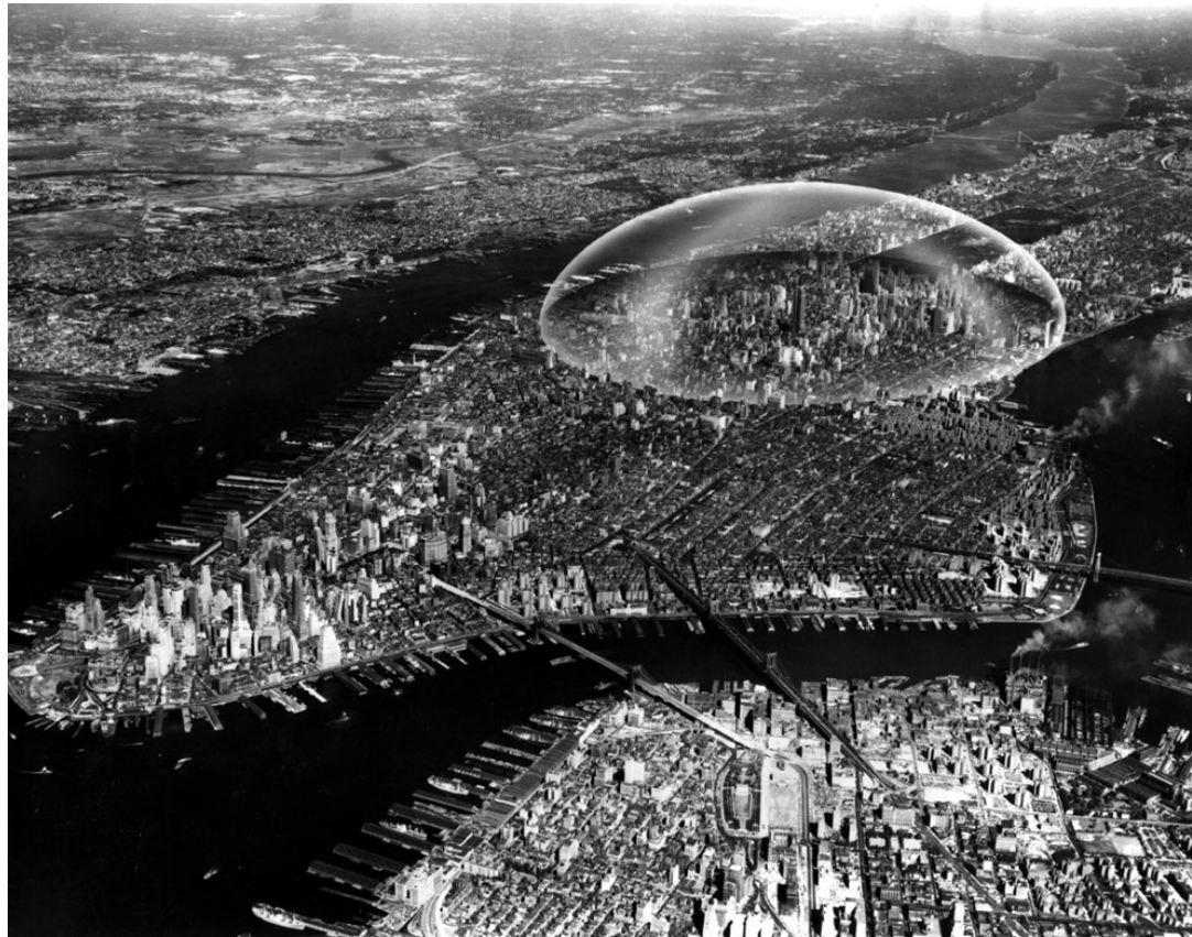
Figure 1.7- 'Dome over Manhattan' by Buckminster Fuller (1960). Buckminster Fuller's proposal of placing a glass geodesic dome two miles in diameter over Midtown Manhattan in order to create a perfectly climate-controlled environment within the city and reduce air pollution.
