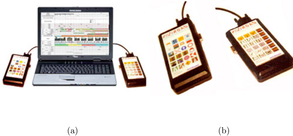
Figure 2.1: (a) VIZIROAD is a system used by road surveyors to track road quality. (b) Various keys on the available keypad correspond to different road defects [32].
