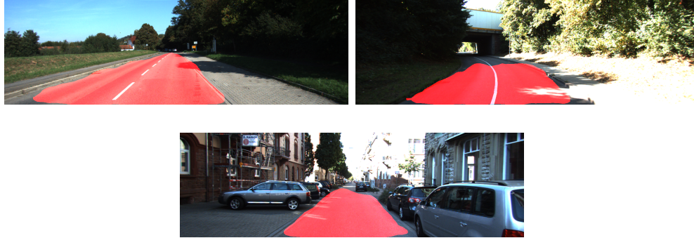
Figure 4.1: Sample segmentation results of our basic method (with the spatial prior) on testing images from the KITTI Dataset. The predicted road segmentation is overlaid in red. This method exhibits invariance to shadows and other road artefacts, however it does not precisely adhere to road boundaries.
