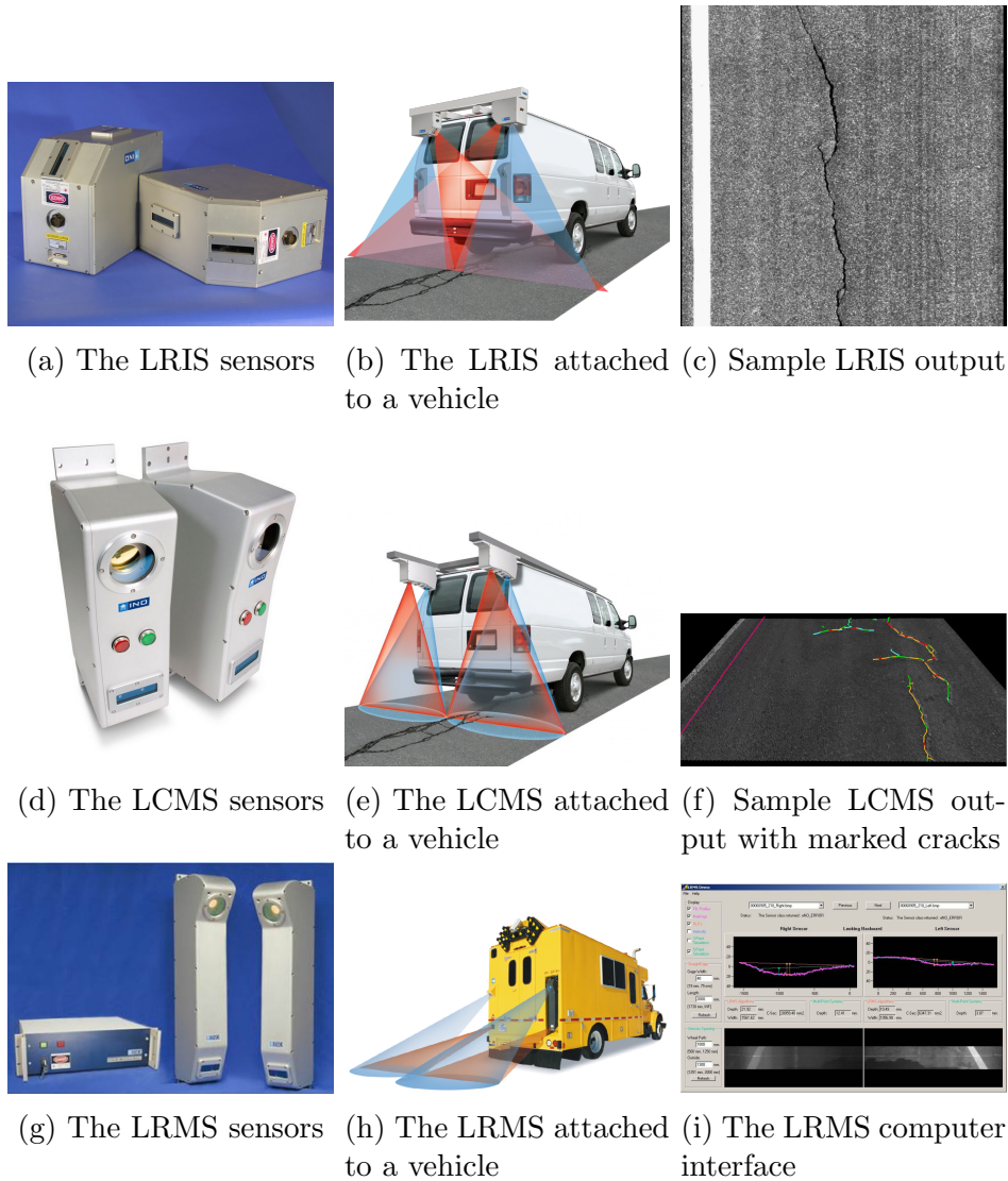
Figure 2.3: The LRIS (a,b,c) captures high resolution 2D road data in a four meter-wide range, it utilizes line lasers to eliminate undesirable illumination effects. The LCMS (d,e,f) uses a combination of cameras and lasers to capture textured 3D road data. It is an all-encompassing road defect sensor that includes proprietary crack detection libraries that annotate cracks based on severity by utilizing the measured crack depth, and can detect rutting, potholes and other defects. The LRMS (g,h,i) uses lasers to detect road rutting specifically. Photos courtesy of [62]
