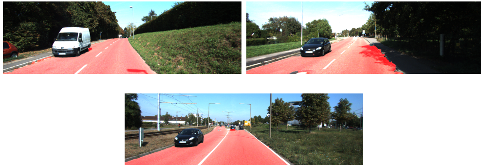
Figure 4.2: Sample segmentation results of our improved method on testing images from the KITTI Dataset. The predicted segmentation is also overlaid in red. This method adheres to natural boundaries more than the basic method, but can be fooled by shadows and other edges.
