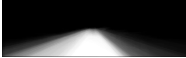
Figure 3.4: The spatial prior is generated for the road class by calculating the times a pixel adopted the road class in the training set. The segmentation relies on the prior to weight its Gaussian windows based on the location they are applied to.
