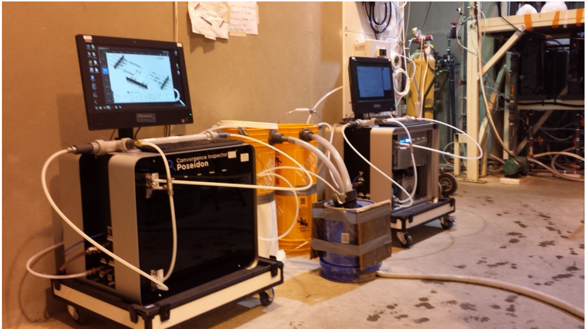
Figure A-3 – Membrane test units used for the membrane fouling experiments.
