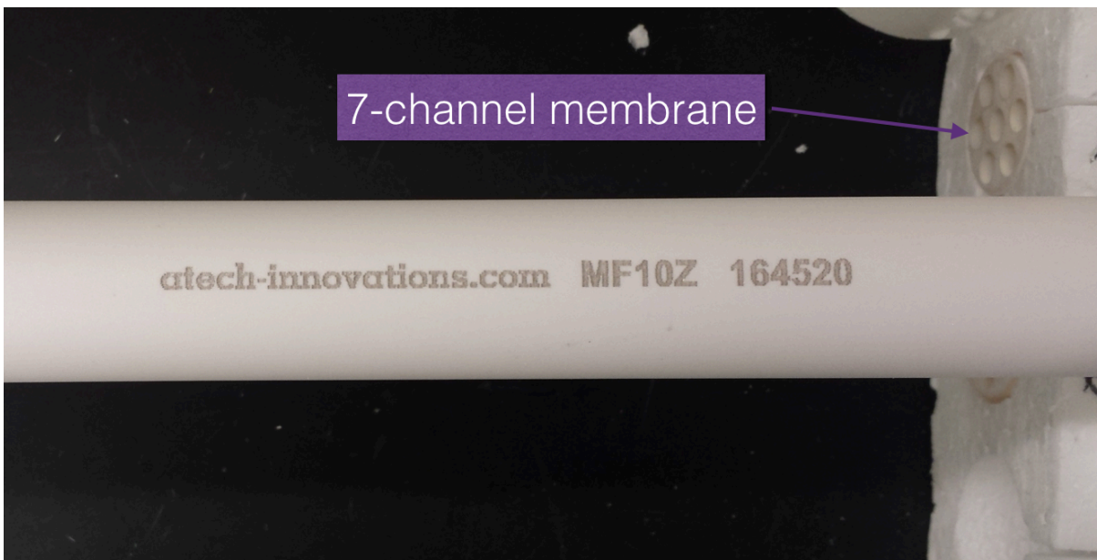
Figure A-4 – MF ceramic membrane manufactured by Atech-innovations, Germany.
