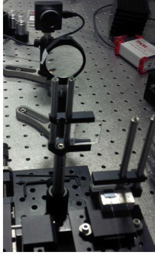
Figure 5.5: The crossed cylindrical imaging setup for the waveguides output facet.
