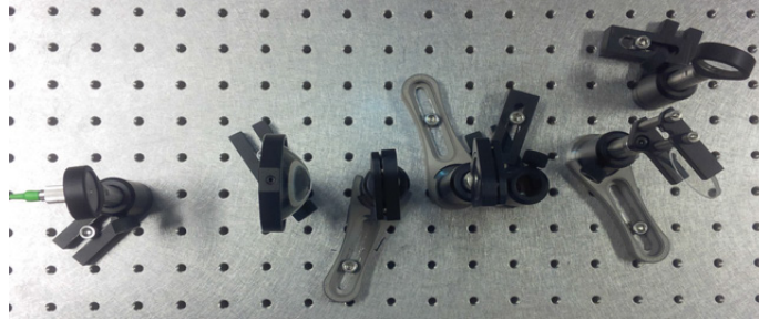
Figure 5.10: The bench-top setup of the designed spectrometer.
