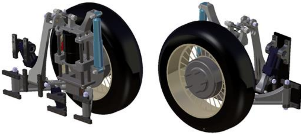
Figure 5-2: Final design of the corner module.
