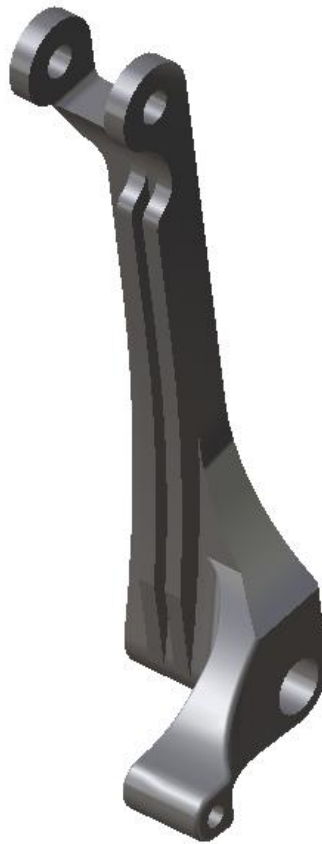
Figure 5-10: Camber link. Two ribs along the length of the link increase its bending stiffness.
