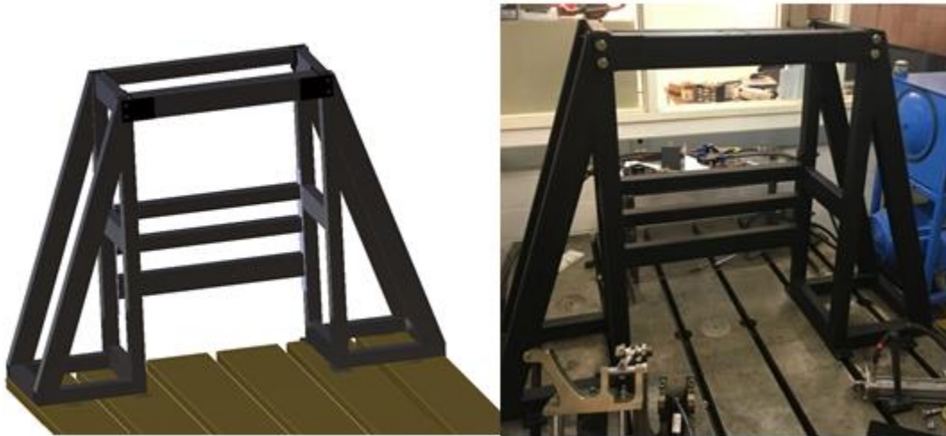
Figure 6-8: Gantry test structure for the corner module. This piece represents the chassis of the vehicle where the corner module is installed on.
