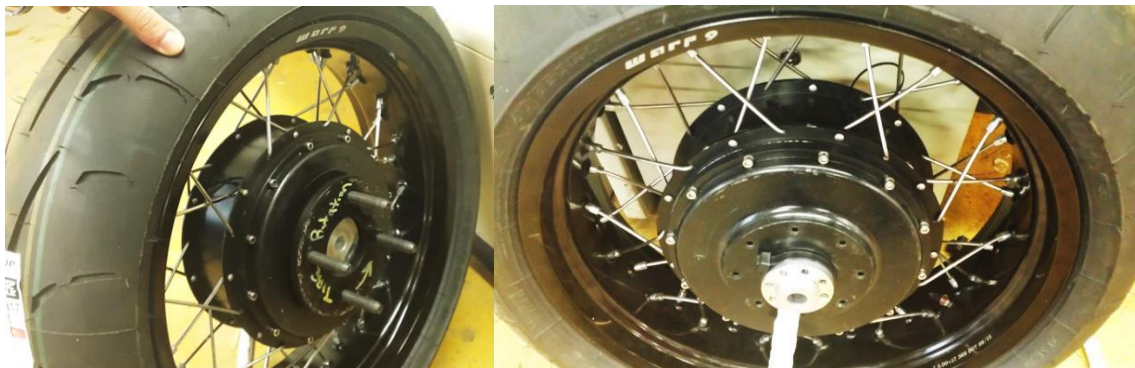
Figure 6-7: In-wheel motor is connected to the rim by spokes.
