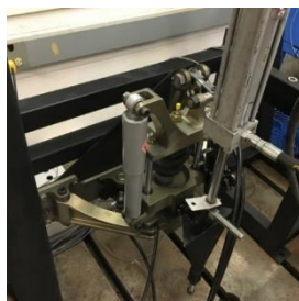
Figure 6-20: Corner module on the test stand in its nominal position at zero steering and zero camber.
