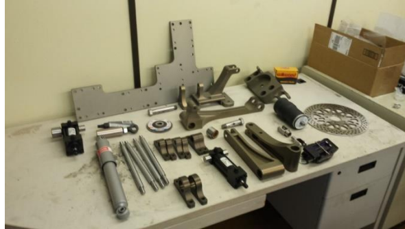
Figure 6-4: Components of the corner module before assembly.
