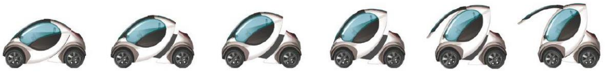
Figure 2-5: Hiriki foldable chassis [12]
