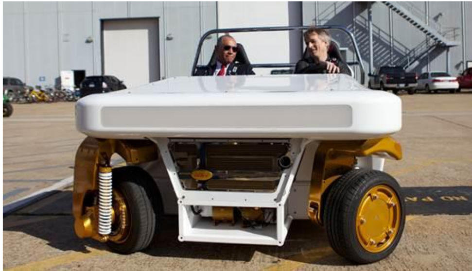
Figure 2-11: NASA MRV wheels can rotate 180 degrees which provides ultimate stability and maneuverability for the vehicle [14]
