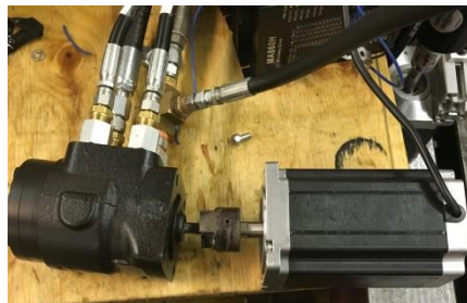
Figure 6-17: Stepper motor driving the steering valve.
