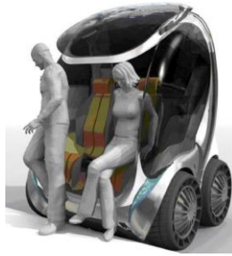
Figure 2-6: Hiriki folds for parking purposes [12]
