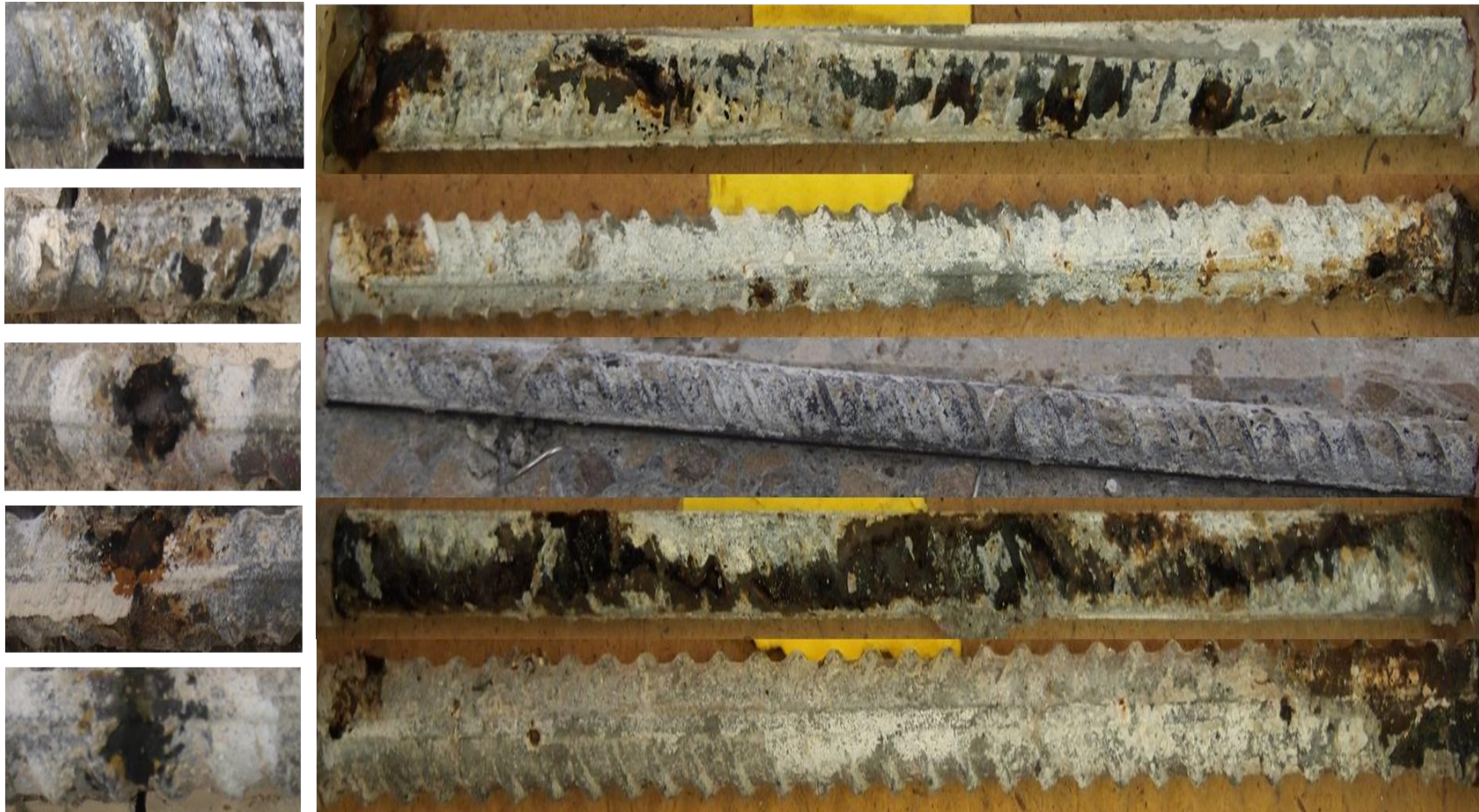
Figure E2.1.1: Exposed surface (to concrete crack) of transversely- (left) and longitudinally- (right) cracked C1 steel specimen
