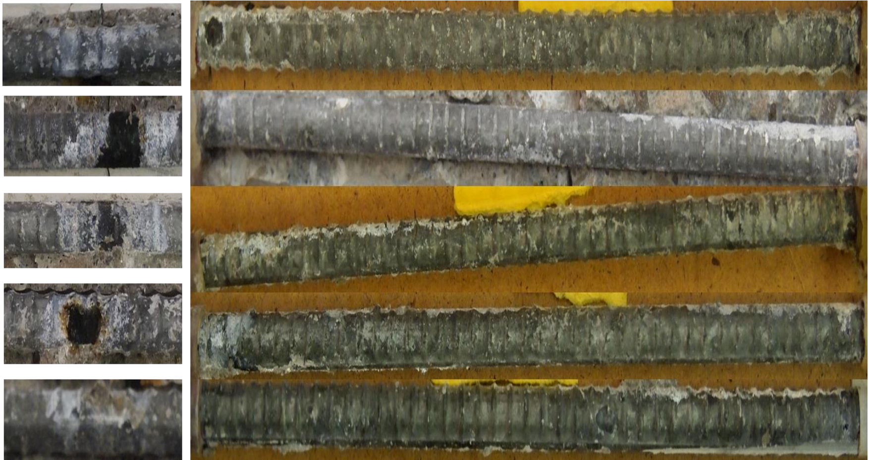
Figure E2.5.2: Non-exposed surface (to concrete crack) of transversely- (left) and longitudinally- (right) cracked C1 steel specimen 1 to 5.
