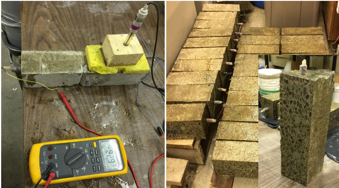
Figure 3-8: Measurement of corrosion potential before exposure to brine (left); and epoxy of all but cracked side of the prisms (right). Closer view of individual prism (insert).
