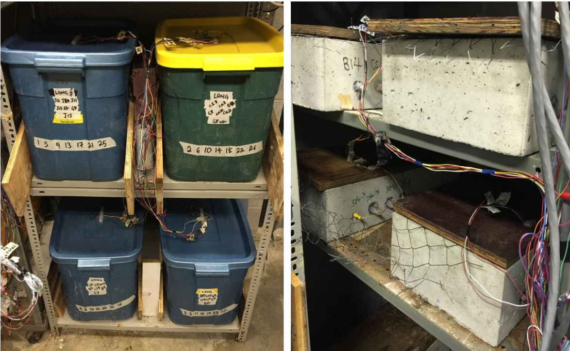
Figure 3-10: Cracked specimens closed in tubs (left), and sound beams closed with plywood (Right).
