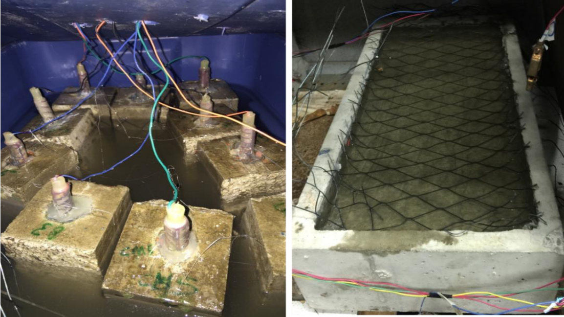
Figure 3-9: Specimen exposure to brine solution. Cracked specimens are placed in tubs containing brine solution while ponding well is filled with brine.
