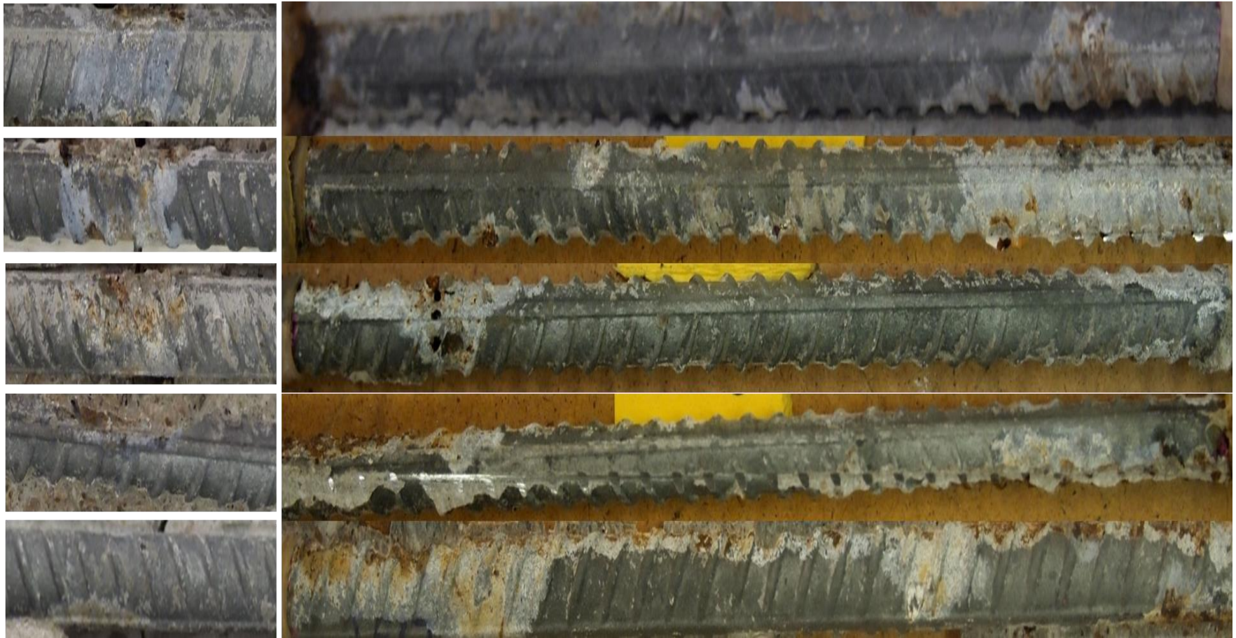
Figure E2.2.2: Non-exposed surface (to concrete crack) of transversely- (left) and longitudinally- (right) cracked C2 steel specimen 1 to 5.
