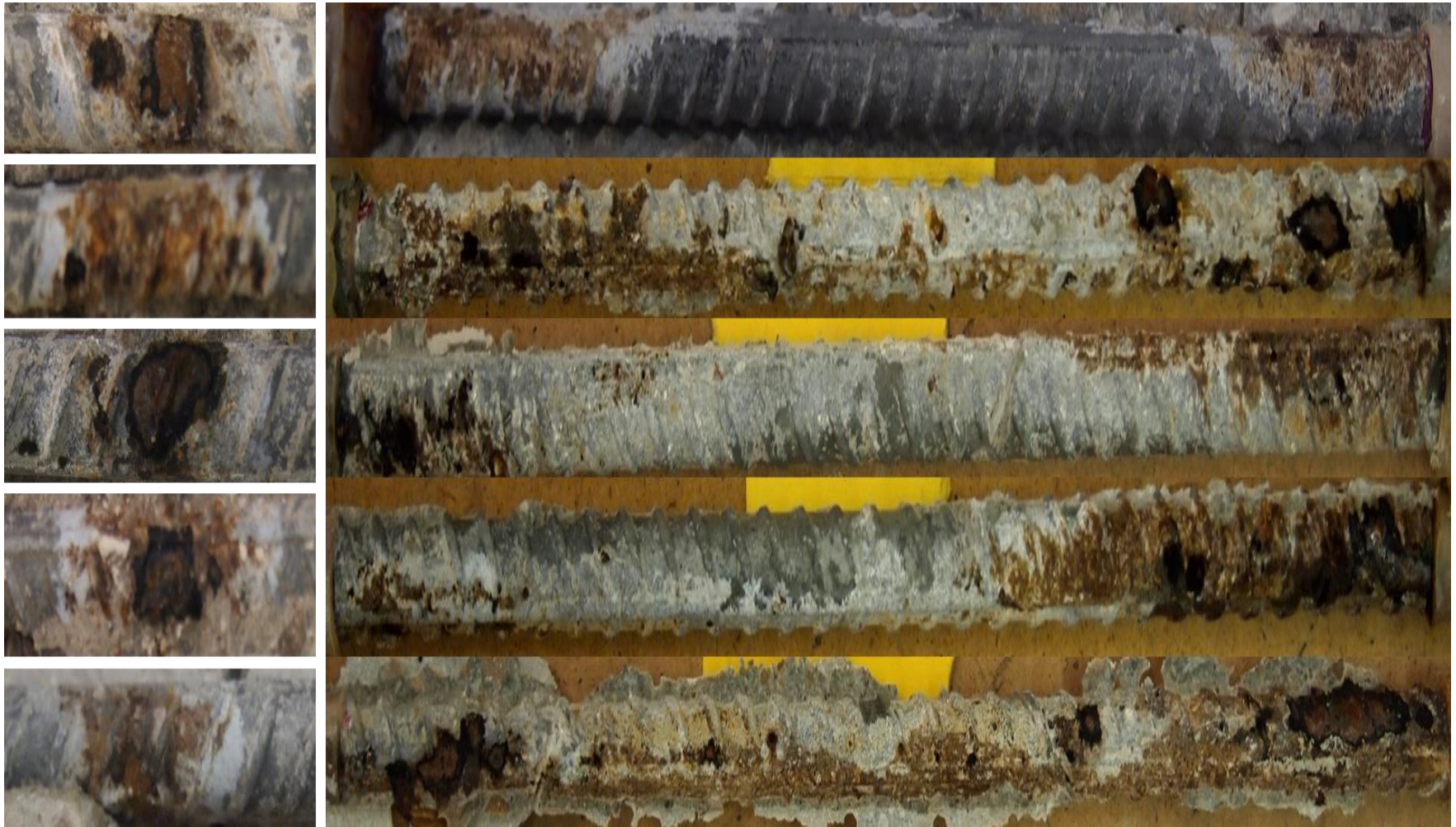
Figure E2.2.1: Exposed surface (to concrete crack) of transversely- (left) and longitudinally- (right) cracked C2 steel specimen
