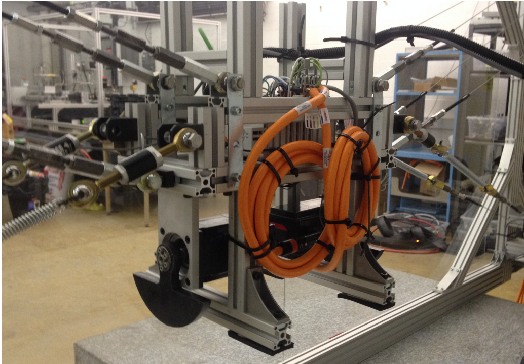
Figure 5.15: Platform mounted pendulum actuator prototype
