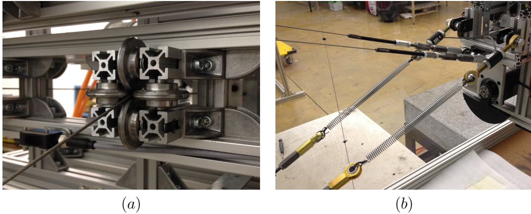
Figure 5.3: (a) Cable rollers (b) Cable-platform spherical joints
