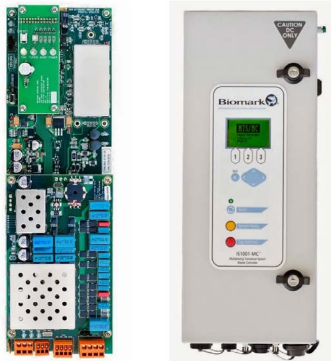
Figure 45 BioMark IS1001 Reader Module
