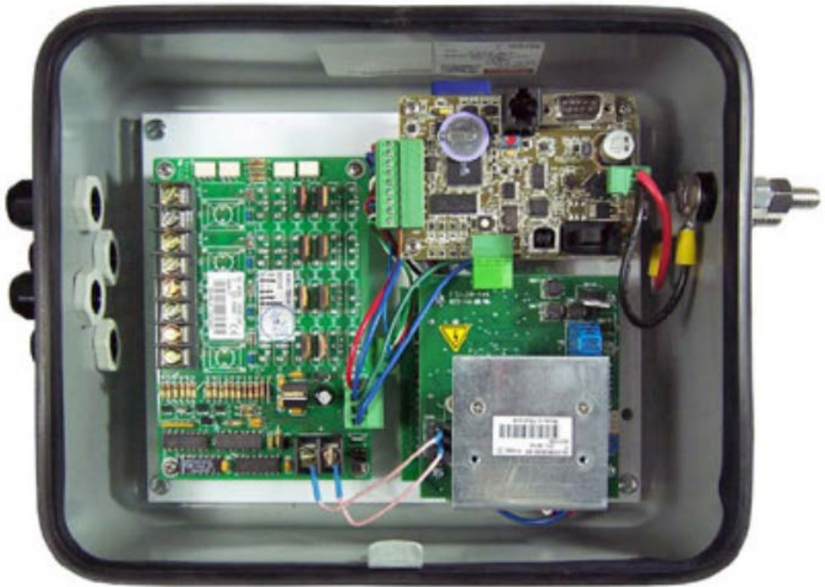
Figure 46 Oregon RFID Multiplexer with Control Module, RF Module, and Data Logger
