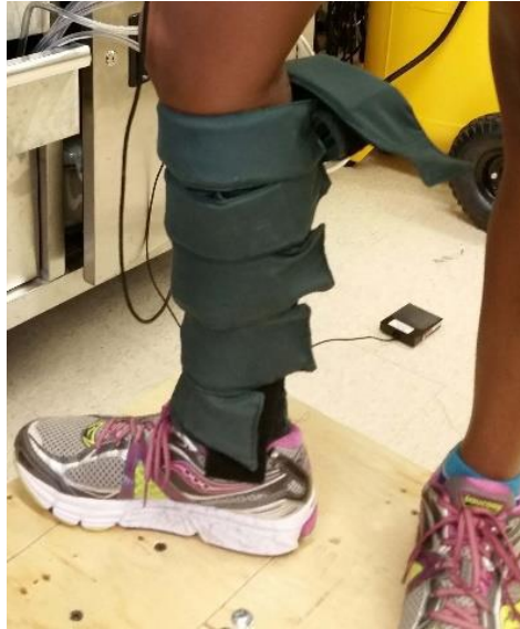
Figure 2-3. Pneumatic active compression system with 5 compression cuffs.
