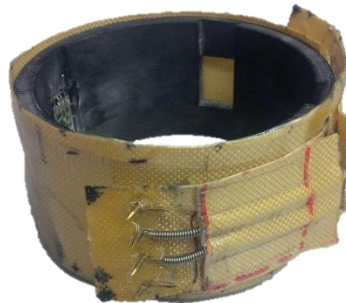
Figure 3-3. Soft belt mechanism with attached compression springs.
