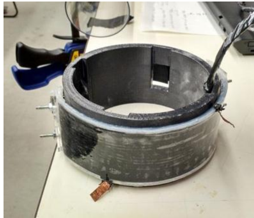
Figure 4-4. DE connected around test bed without belt mechanism.
