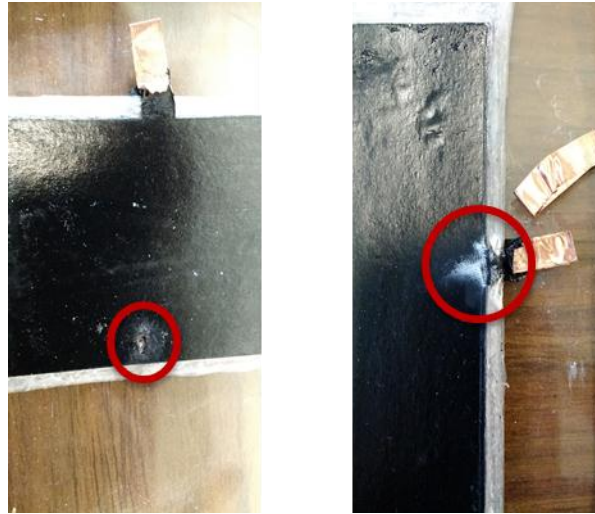
Figure 4-15. Actuator failure locations. From left to right: A12-50W, A30-50W.
