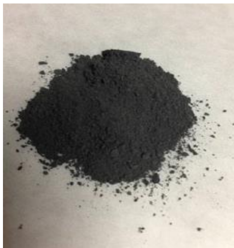
Figure 2-1 Dark grey graphene/EC powder [Reprinted with permission of Elsevier] [41].
