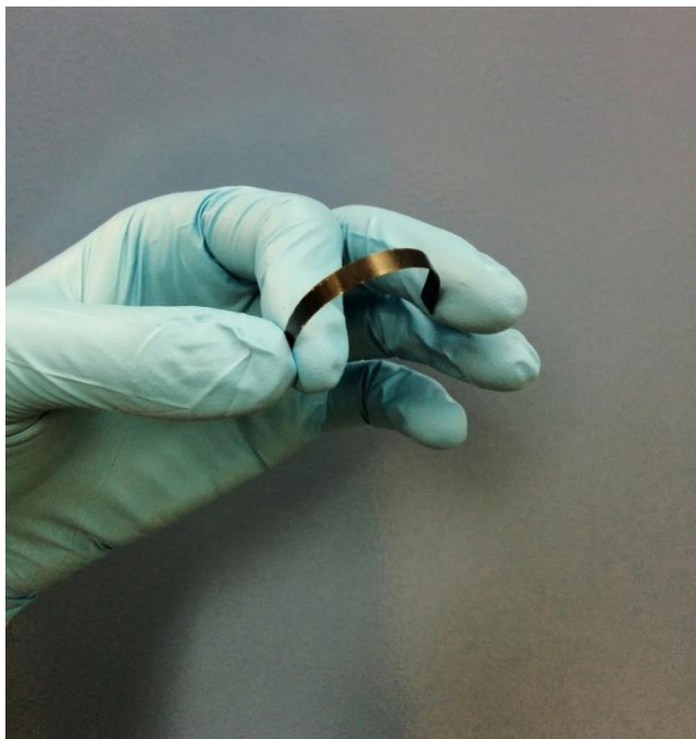
Figure 2-8 Graphene paper samples cut in rectangular strips.
