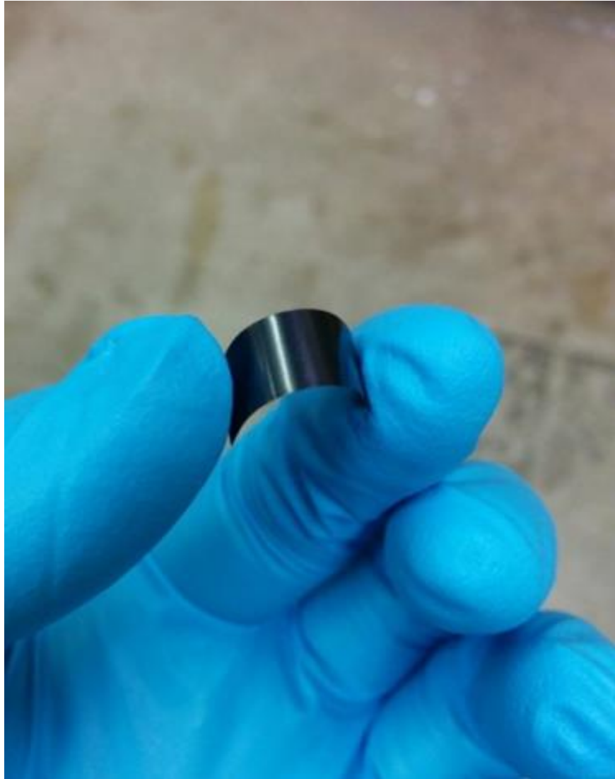
Figure 3-4 Graphene paper sample for electrical resistance experiment.
