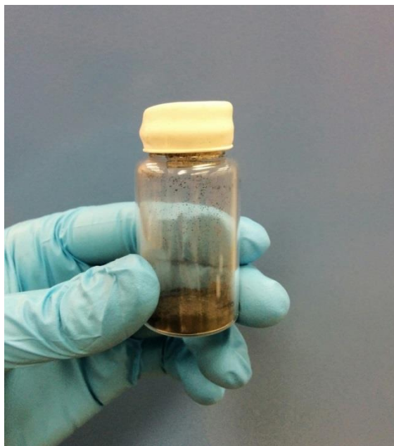
Figure 2-10 Graphene/EC powder vial with a rolled over septa.
