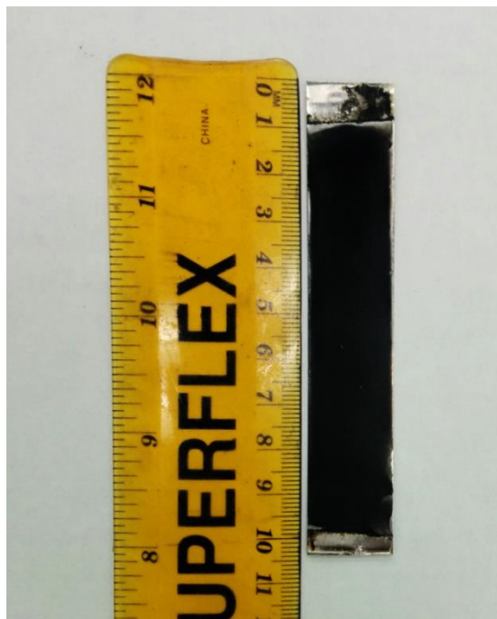
Figure 2-17 Ni/Graphene electrode for supercapacitance test.
