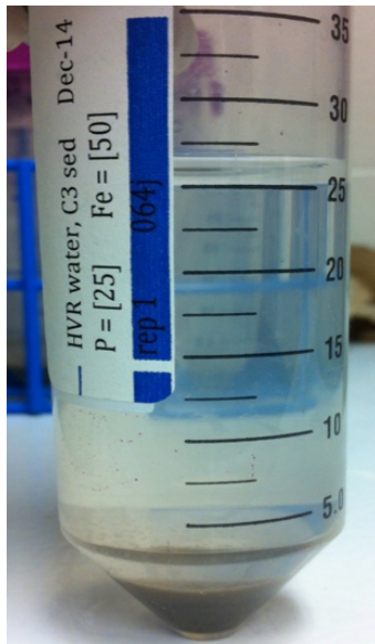
Reservoir Water + sediment P = 25 \mu\text{g/L} . \text{FeCl}_3 = 50 \text{ mg/L}
