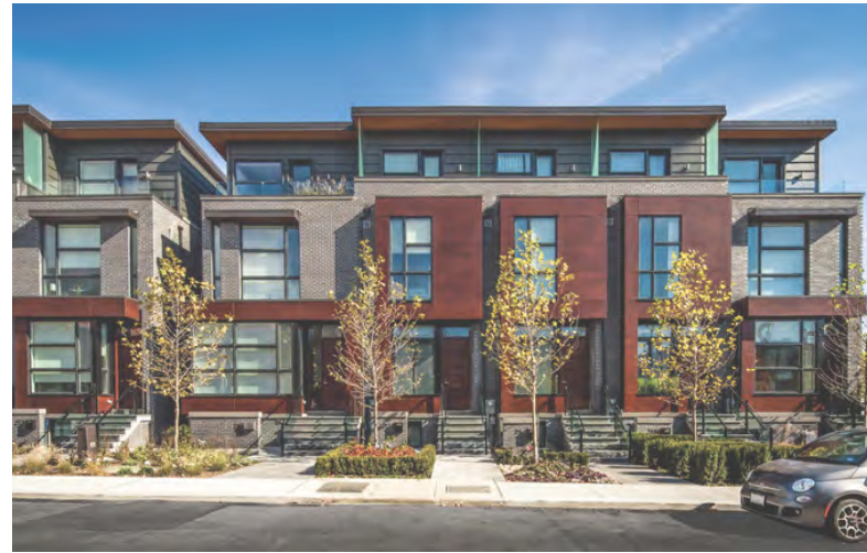
fig 3.111 Street view of the townhouse units having raised units and four metre setbacks from the sidewalk edge.
