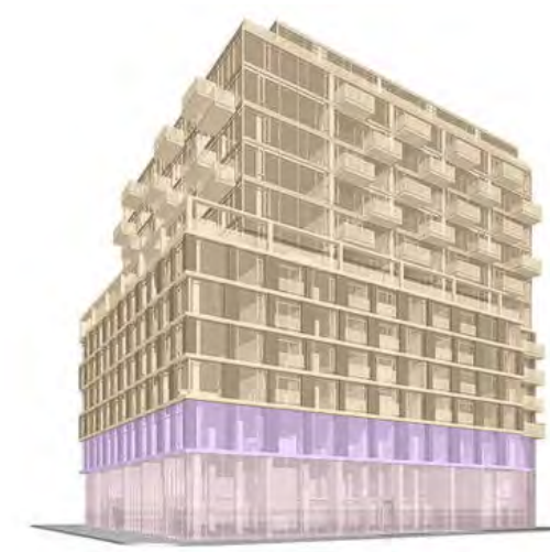
fig 3.86 East elevation land-use diagram showing each land-use's location and varied floor-to-floor height.
