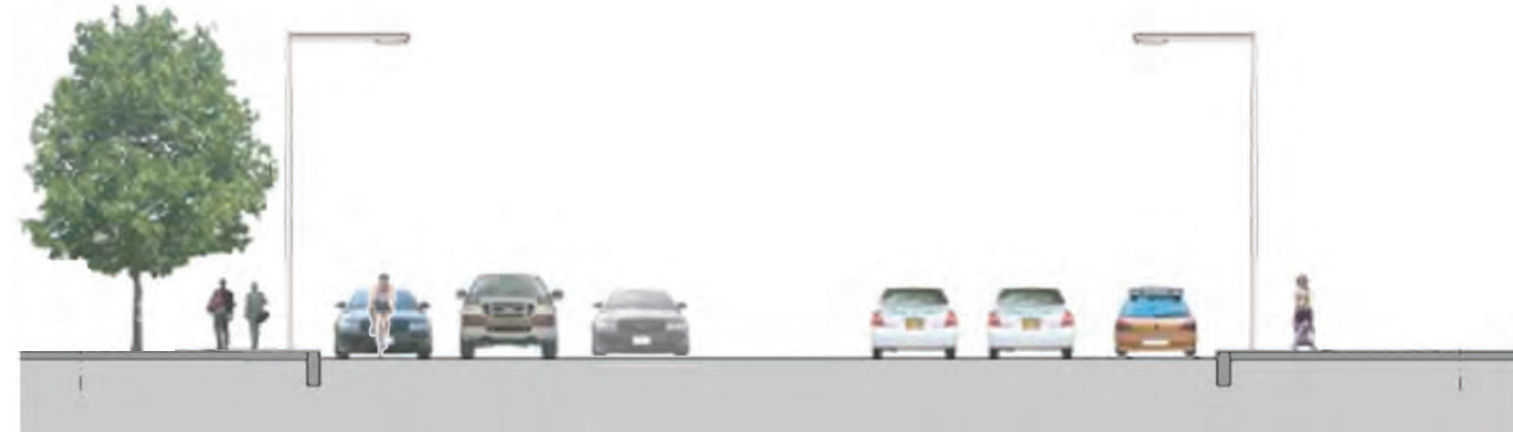
fig 3.23 Typical cross-section of the Golden Mile's existing street having a 36m right-of-way.
