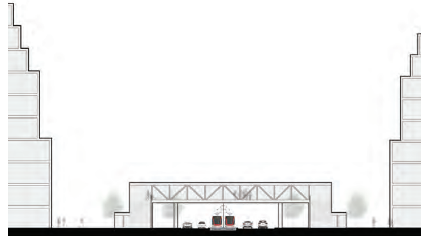
fig 5.41 Freestanding pedestrian bridge street crossing option.
