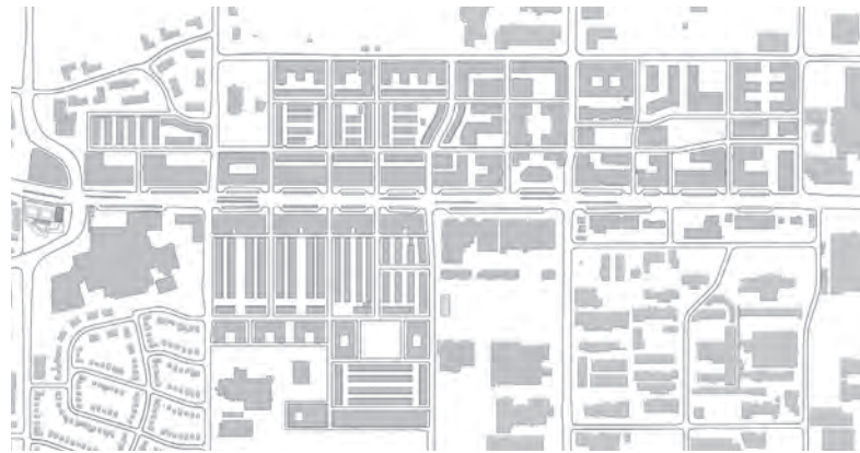
fig 4.25 Proposed Built-Block diagram shows the area's proposed intensification with a significant increase in lot coverage and buildings that are built to plane addressing the street well.
