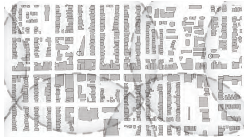
fig 5.86 Bloor-Bathurst District Transit Shed diagram shows 500m walking sheds of the Bloor subway, Bathurst streetcar, and Spadina streetcar. Together, these three transit corridors cover the entire district easily. The mix and structure of land uses found in the district, though simplistic, attract people to the area to live, shop, and be entertained. This influx of people to the district increases the support for transit, commercial properties, and for the creation of an activated urban area.
