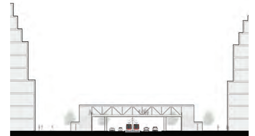
fig 3.11 Freestanding pedestrian bridge street crossing option.
