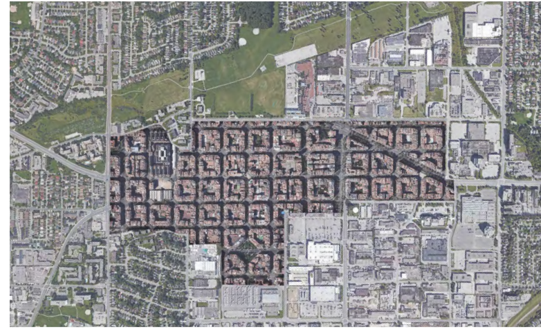
fig 4.2 Aerial image of Barcelona's Eixample blocks superimposed on the Golden Mile comparing scale. The area of the Golden Mile's proposed reurbanization is 98 hectares. Currently, this area is comprised of commercial and employment uses (with no dwelling units). The Barcelona blocks have approximately 4.7 floor-to-area ratio, with a density of 359 people and 230 dwelling units per hectare (employment densities were not available). 76 Applying Barcelona's Eixample density (359 people and 230 units per hectare) to the Golden Mile would result in a population of approximately 35,200 people with 22,500 dwelling units. In order to accommodate future population and employment growth, help to support transit, and make more the area more enjoyable, the Golden Mile requires a vast transformation from its current state (figure 4.3).
