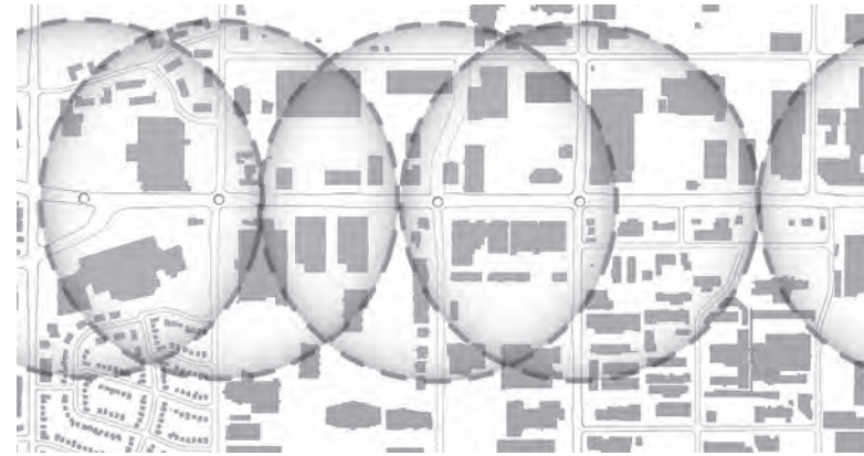
fig 4.26 The existing Transit Shed diagram shows the number of buildings within a (as the bird flies) 500m radius of future LRT nodes.
