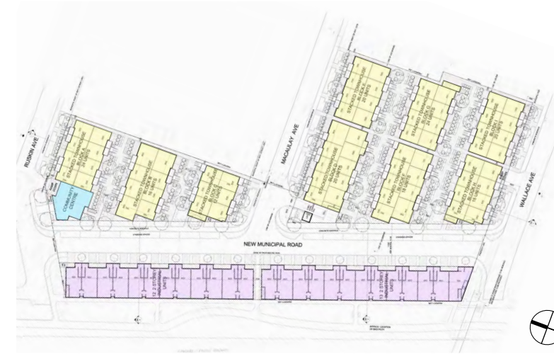
fig 3.102 Site plan land-use diagram showing stacked back-to-back residential townhouses, light industrial units, and community centre.
