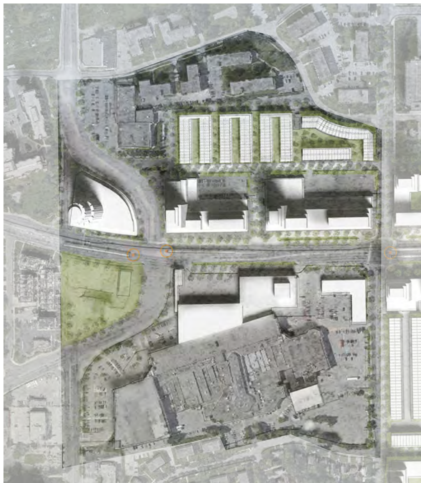
fig 4.51 Precinct One's Plan View Render shows the intersection shift, the mall's proposed addition, and the precinct's proposed massing.
