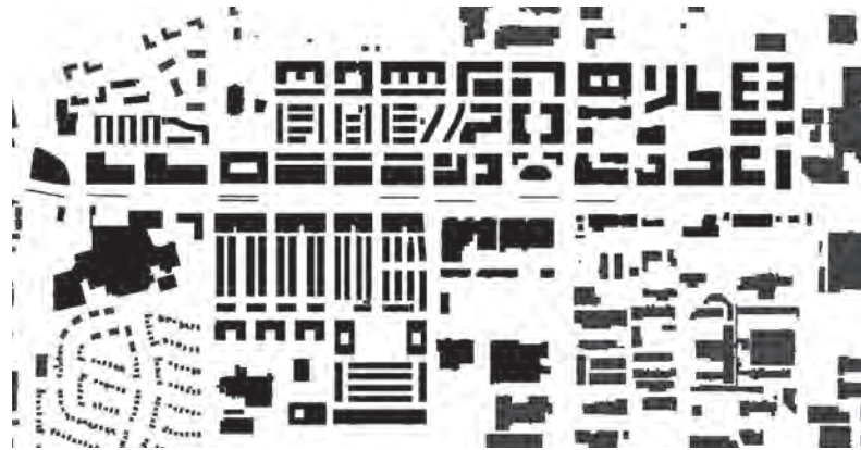
fig 4.23 Proposed Figure-Ground diagram shows a clear transformation of the district's morphology as building sizes are reduced while built intensity and density are increased.
