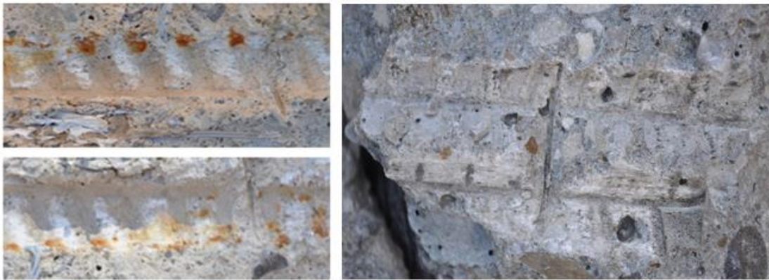
Figure 4.18 The interface of the concrete ahead of the steel bar ribs for the FRP wrapped specimens
