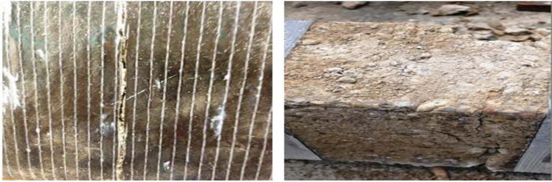
Figure 4.17 Typical failure mode for the FRP wrapped specimens
