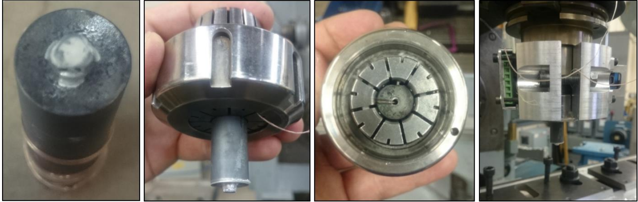
Figure 25: Tool-embedded thermocouple setup
