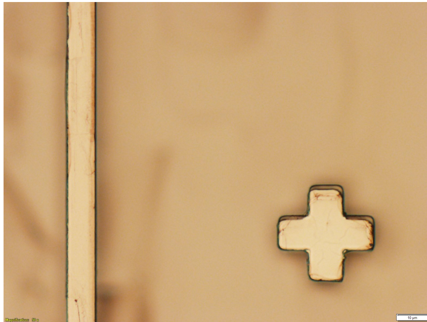
Figure 2.14: Chromium on SU8 core obtained using the procedure depicted in Figure 2.13.
