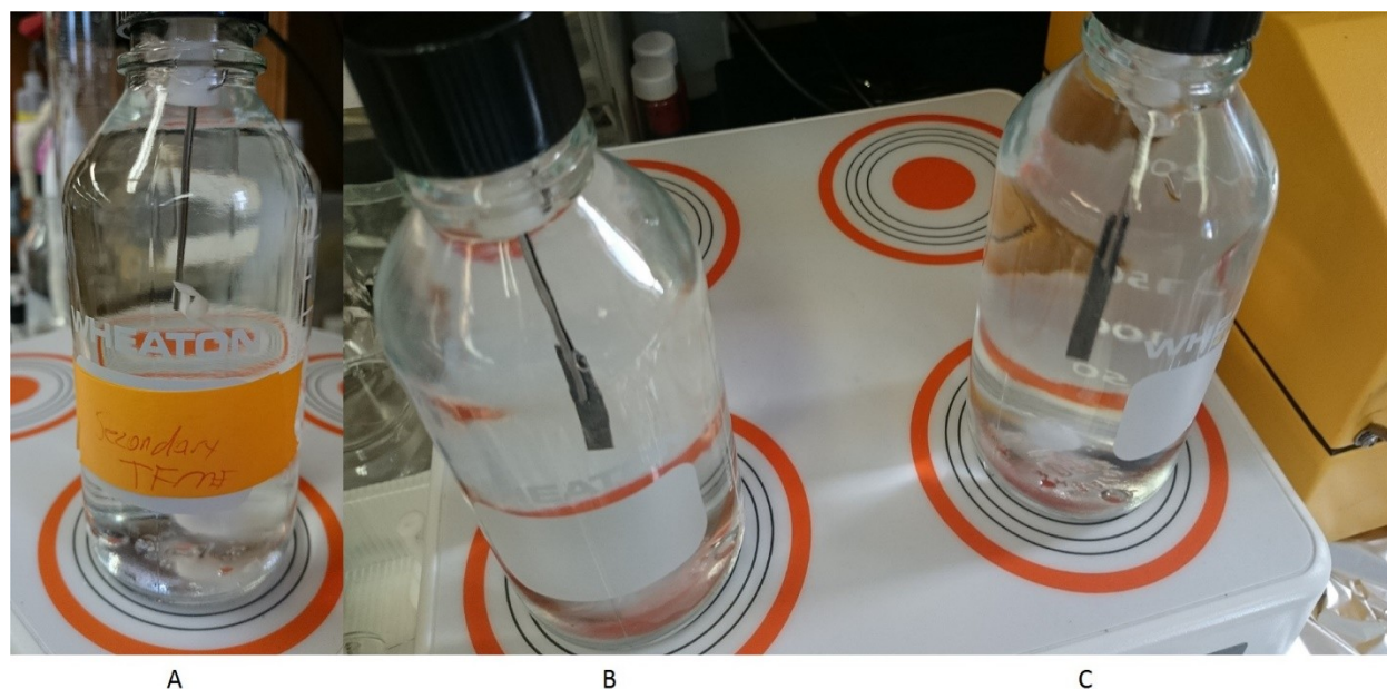
Figure S.4. Direct immersion sampling of pesticides at 1000 rpm with: (A) a 2 cm long, unsupported DVB/PDMS membrane; (B) a 2 cm long DVB/PDMS/Carbon mesh supported membrane; (C) a 4 cm long DVB/PDMS/Carbon mesh supported membrane.
