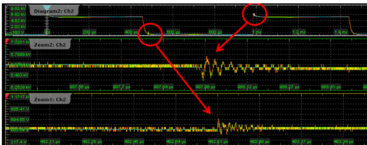
Figure 4.7. Comparing the measured PD pulse polarities at rise and fall times.
