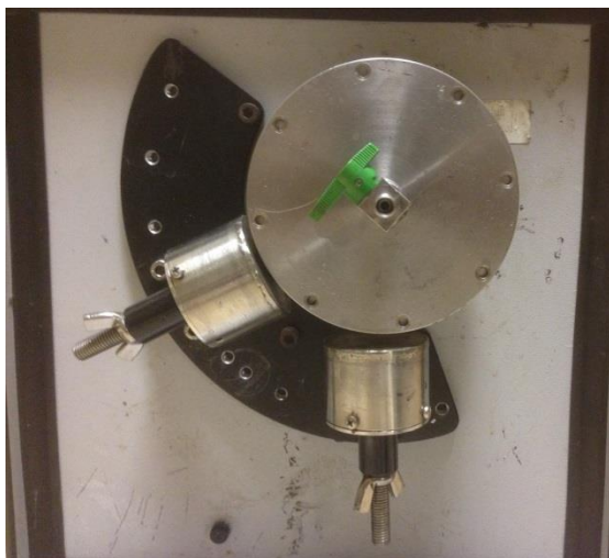
Fig. 3-1 An optical photo showing the angular position of magnets at 6 and 8 o'clock (IMP 68) for ball milling in the Uni-Ball-Mill 5.
