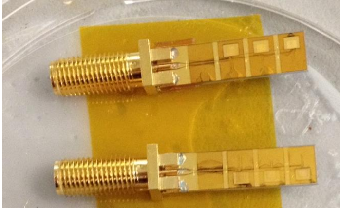
Figure 5.16: The three sensor array on the rigid RFID platform. These RFID arrays are the same size as those shown in Figure 5.2.
