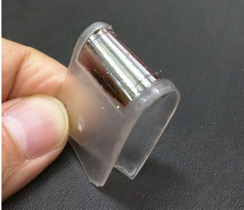
Figure 6-9: CMUT after thinning can be curved.
