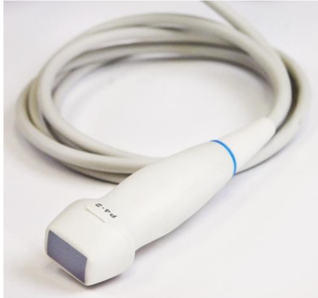
Figure 2-5: A Verasonics medical phased-array probe
