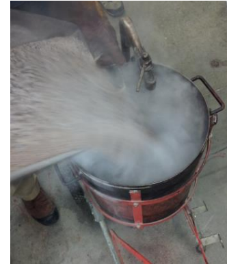
(d) Adding heated aggregate blend to the mixer drum
