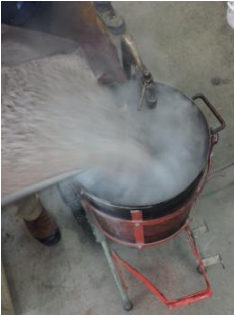
(a) Adding heated red granite aggregate blend
