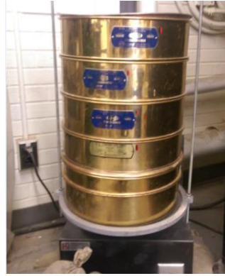
(b) Sieving oven-dried aggregate
