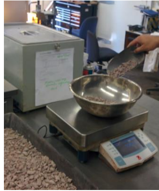
(c) Batching the aggregate blend according to the JMF
