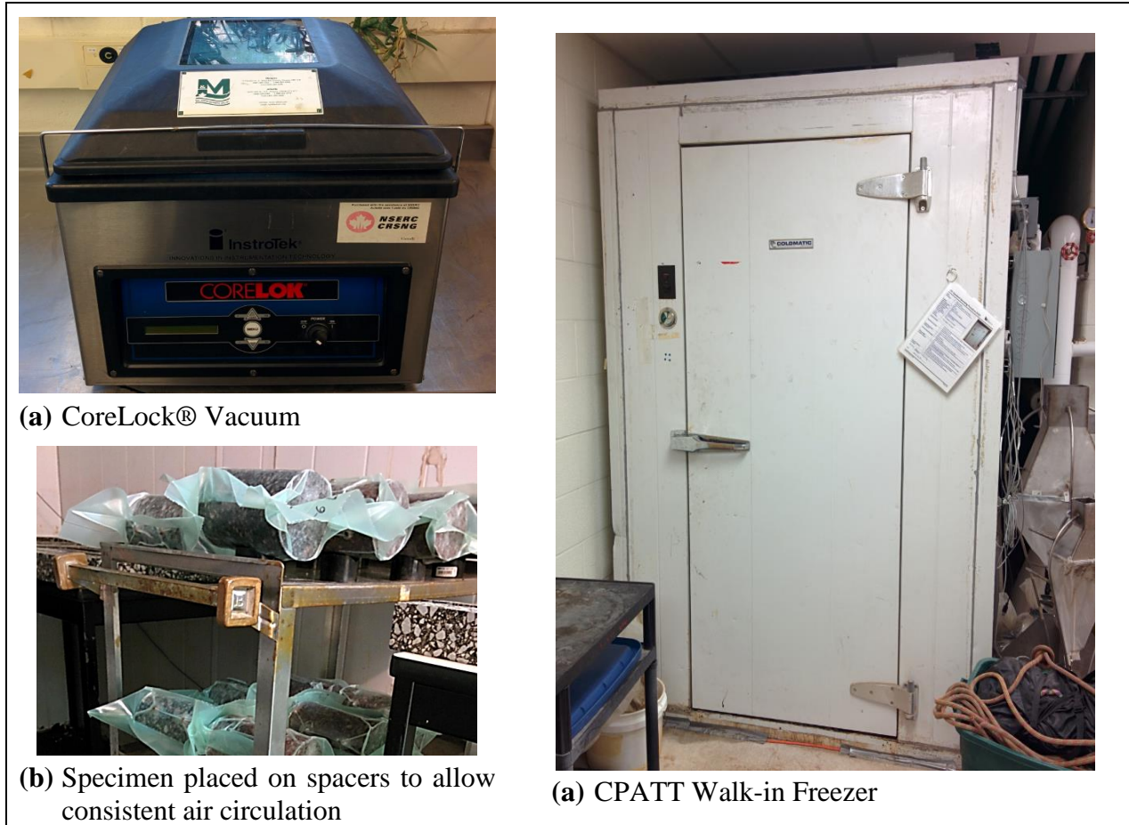
Figure 3-24 CPATT Equipment Used for Freeze-Thaw Durability Test
