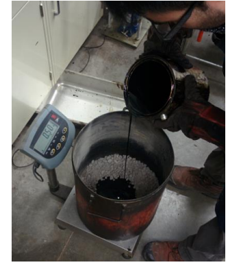
(e) Adding required amount of asphalt binder treated with warm-mix additive
