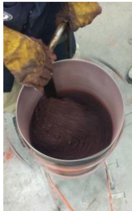
(d) Mixing for 90 seconds to achieve consistent colour and coating
