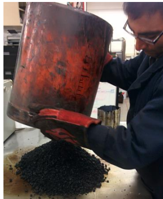
(g) Mixture discharging on flat, non-abrasive, non-absorptive, and warm surface area
