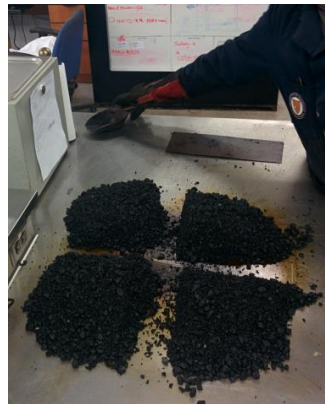
(h) Flattening and quartering with warmed and oil-sprayed tools to obtain desired testing sample size.
