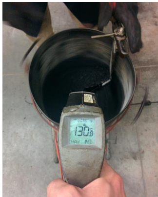
(f) Mixing for 90 as per AASHTO R35 at recommended mixing temperature
