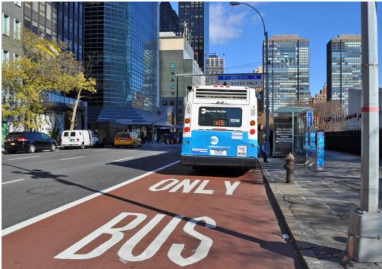
Figure 2-19 Red bus lane on 1 st Avenue in Midtown, Manhattan, United States (Carry, 2012)
