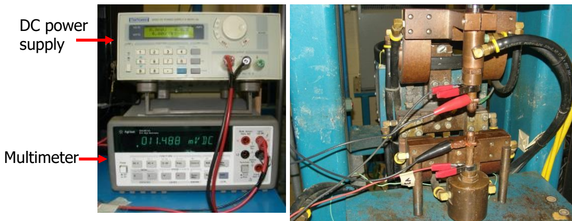
Figure 3-2 Equipment set up for 4-point static resistance measurement
