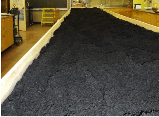
Figure 3-1: Drying frame used for drying GAC
