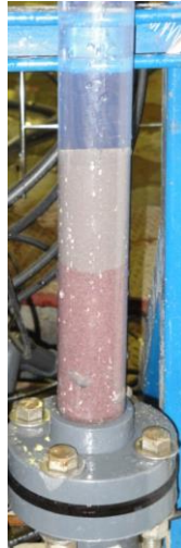
Figure 3-2: Picture of media from two different REC batches installed in a backwashing column. (Media from one batch are grey and media from the other batch are dyed red)
