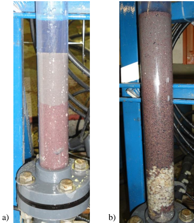
Figure 3-7: Pictures of media from two batches in backwashing column: a) before backwashing and b) after backwashing. (Media from one batch is grey and media from the other batch has been dyed red)
