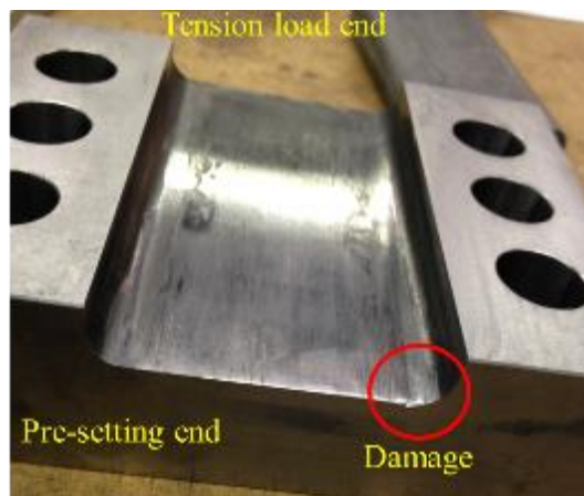
Figure 8.19: Local damage in the barrel of the anchor in the pre-setting end after test for the H13 steel anchor #1 with 55.5 mm wide (full width) wedges.
