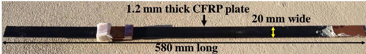
Figure 4.1: A 1.2 mm thick and 20 mm wide CFRP plate.
