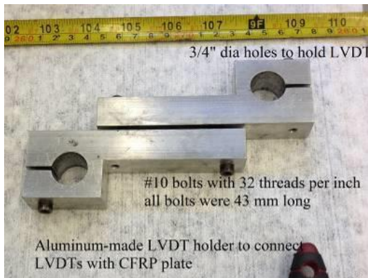
Figure 7.16: (a) Sketch of the LVDT clamp to make it; (b) aluminum-made clamp to hold LVDTs during the tension tests; (c) LVDT clamp with the LVDT together.
