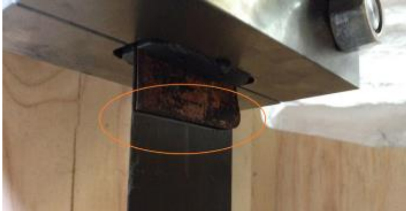
Figure 8.5: CFRP plate did not move from the anchor (as shown in the circle) and wedges slid all the way to the end of barrel during the tension test.
