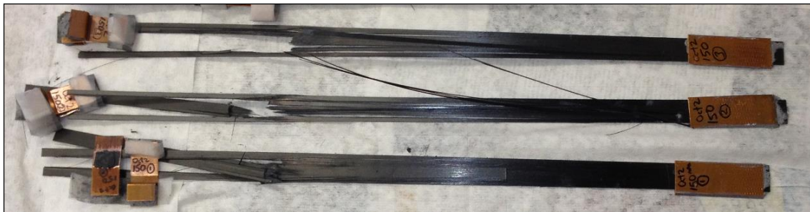
Figure 4.16: The CFRP plates failed in tension after sliding for certain distances – all three samples in this figure have been tested for 150 MPa normal stress.
