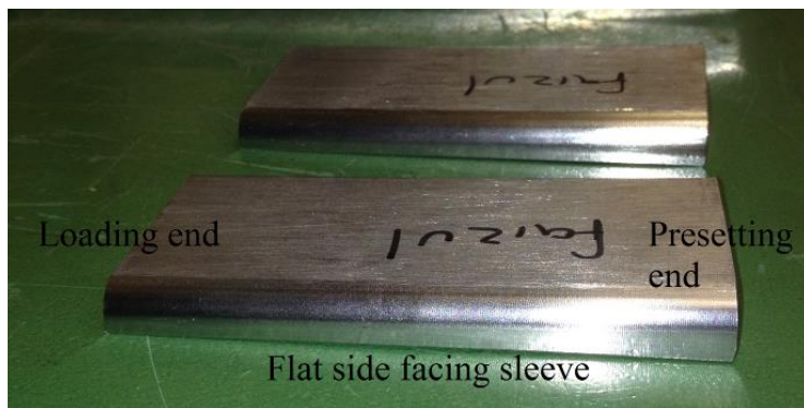
Figure 7.2: (a) Longitudinal profile of wedges, (b) sandblasting of the flat side of wedges.
