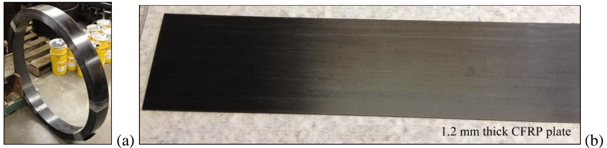
Figure 2.2: (a) A roll of CFRP plate; (b) a 1.2 mm thick CFRP plates.
