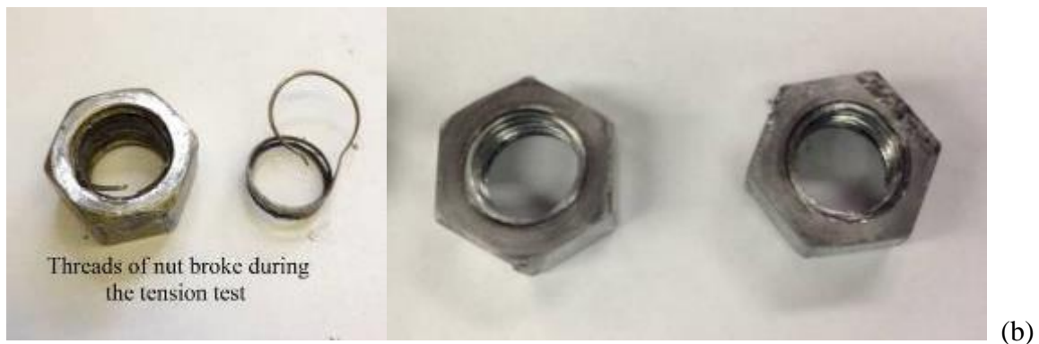
Figure 8.11: Threads of (a) bolts, (b) nuts broke during the tension tests.
