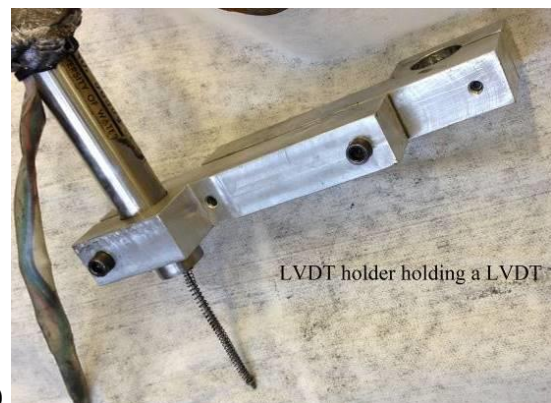
Figure 7.16: (a) Sketch of the LVDT clamp to make it; (b) aluminum-made clamp to hold LVDTs during the tension tests; (c) LVDT clamp with the LVDT together.
