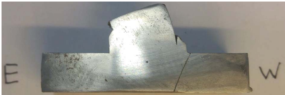
Figure 4-22: Cross-sectional cut made longitudinally through Stud S4 in Specimen C300.
