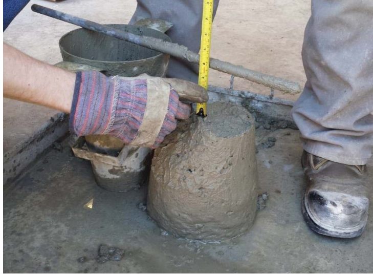
Figure 3-14: 100 mm [4"] slump test results (first cast).
