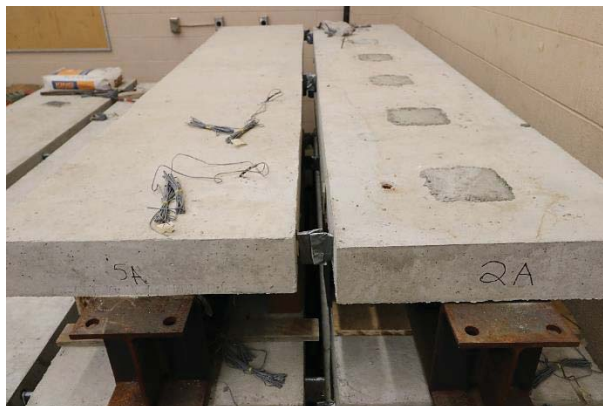
Figure 3-19: Completed specimens: CIP (left), precast (right).
