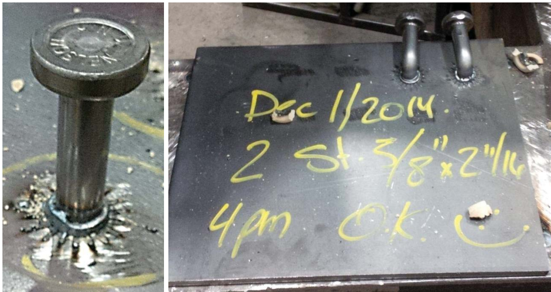
Figure 3-9: A stud after welding (left), and two studs that passed the bend test (right).
