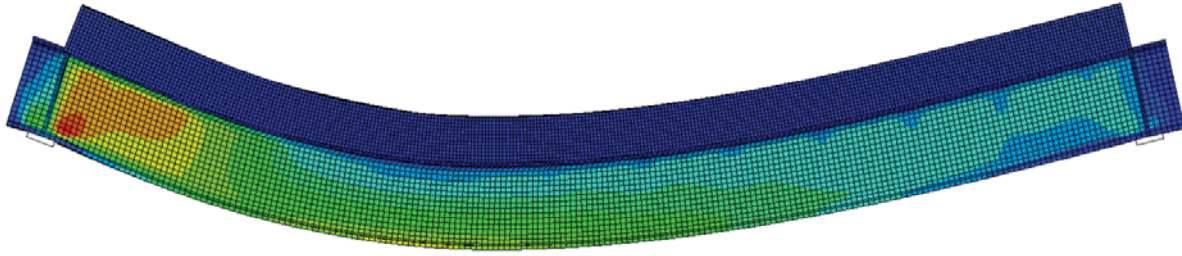
Figure 5-11: Von Mises stress contour plot demonstrating yielding of the web located at the west support at an applied load of 500 kN for the CIP model.
