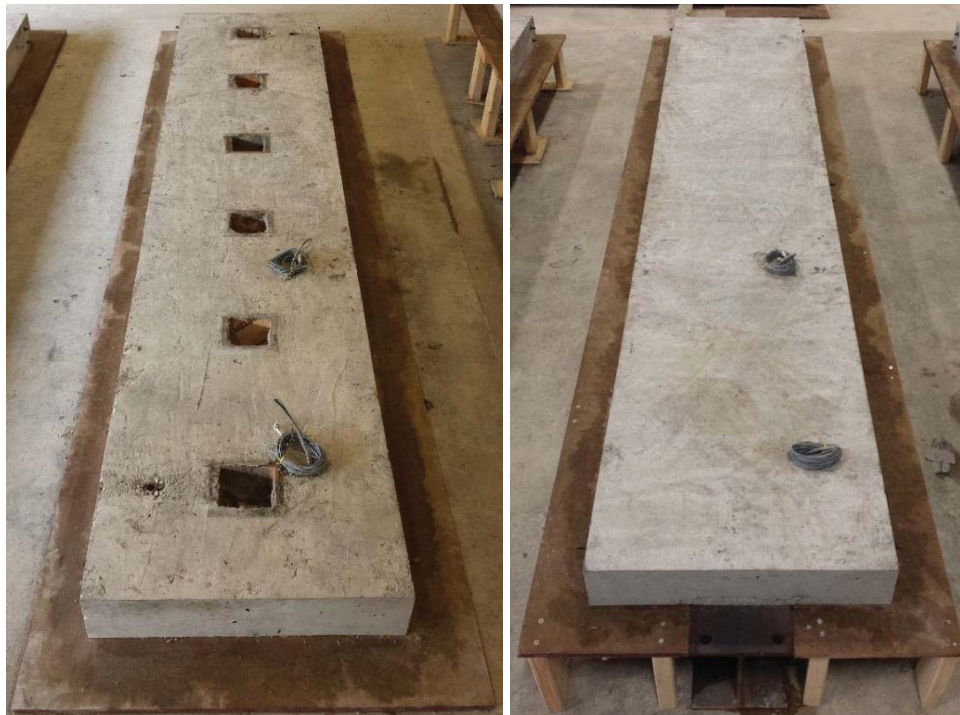
Figure 3-17: After 28 days the formwork was stripped from the slabs.
