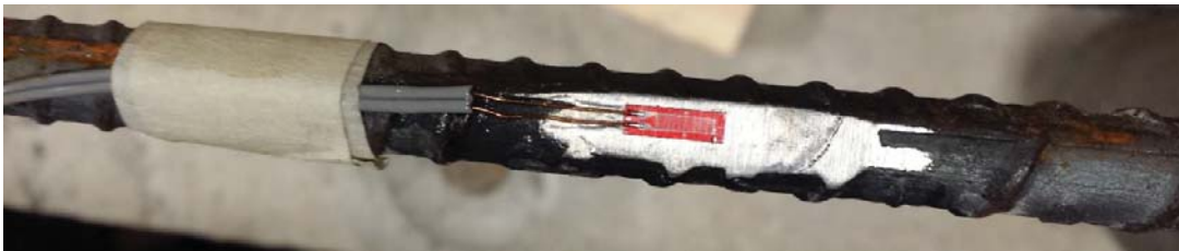
Figure 3-12: Longitudinal reinforcement strain gauge application.
