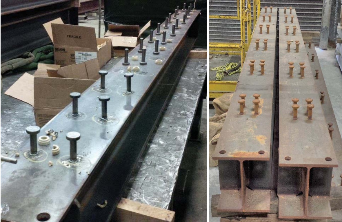
Figure 3-8: Fabrication photos of the CIP and precast steel beams (left and right).
