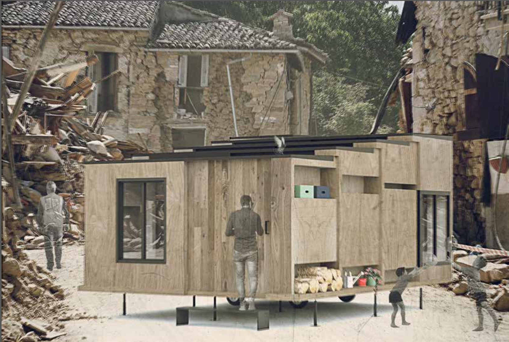
Fig 8.24 These mobile homes can be transported by the disaster survivors to their desired location (close to their own properties) where they can protect their remaining belongings and rebuild their house.
