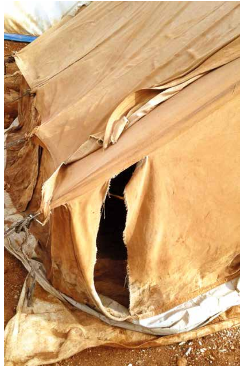
Fig 2.01 Tents can be easily sliced open by sharp objects.
