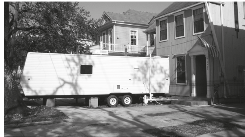
Fig 3.06 FEMA trailers are temporary manufactured houses used by the victims of natural disasters. They include sanitary facilities, kitchen, and furniture. FEMA is designed to operate on grid and can only be installed on properties with running water and electricity. The most critical advantage of these trailers is their mobility which enables them to be installed next to the affected families' property and relocated after permanent houses are reconstructed. 37
