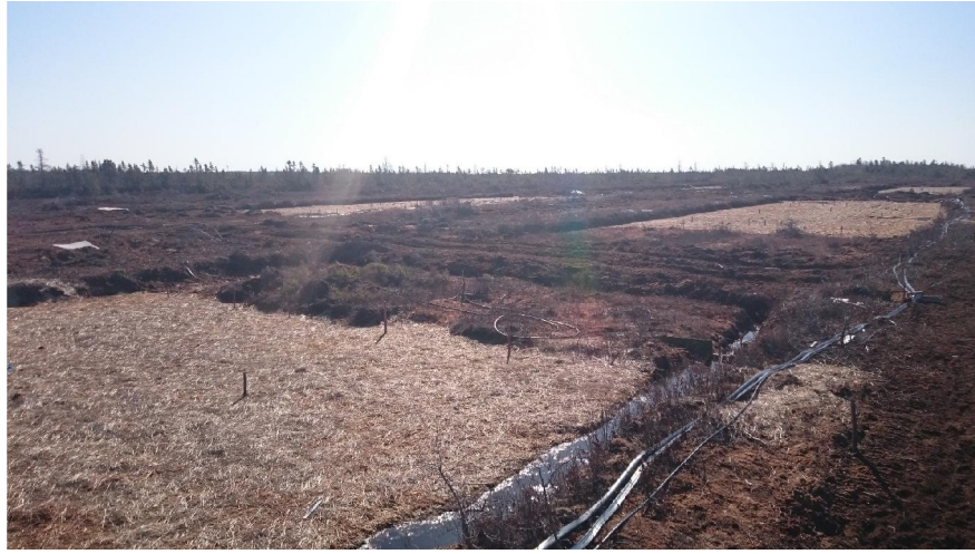
Figure 1-1 Photo (2015) of the straw covered experimental basins within the lowered block-cut trenches.
