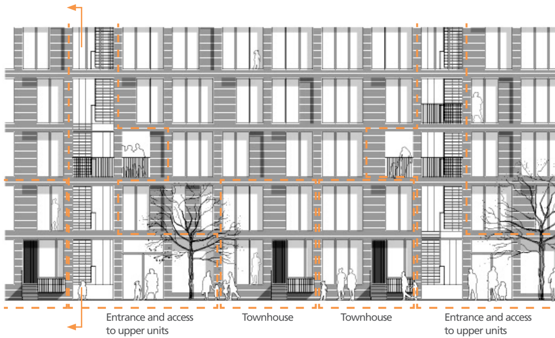
Fig. 3.40. Elevation with breakdown of entrances and circulation areas providing access to units.
