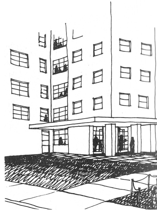
Fig. 3.12. Newman’s analysis of Tilden houses in Brooklyn, New York, where the positioning of windows at the stairwell landings and private units allows for surveillance of the street from the building interior and vice versa.
