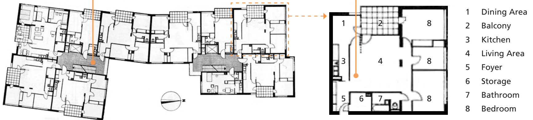
Fig. 3.23. Left - plan of floors 2-7 of the building. Right - plan and room descriptions of a 3-bedroom apartment.
