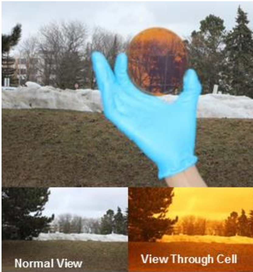
Figure 4-29. Fabricated cell with actual view through the cell (200nm nc-aSi).
