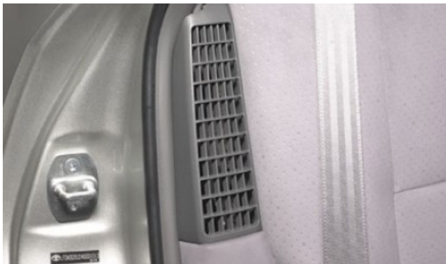
Figure 3.1: Fan vent location. Air is sucked into the battery pack through two vents in the passenger compartment.
