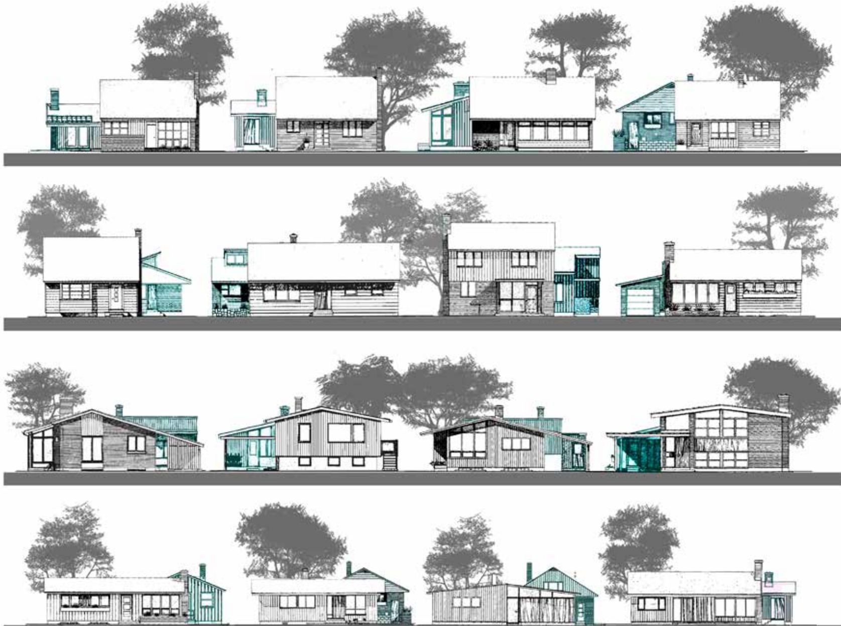
3.30 Typical postwar streetscapes with rear yard coach houses using CMHC Small House Design drawings from the 1958 catalogue.
