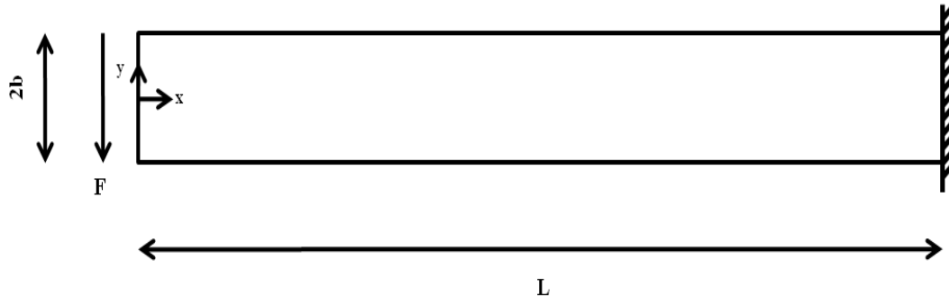
Figure 3.5 Geometry of the elasticity problem
