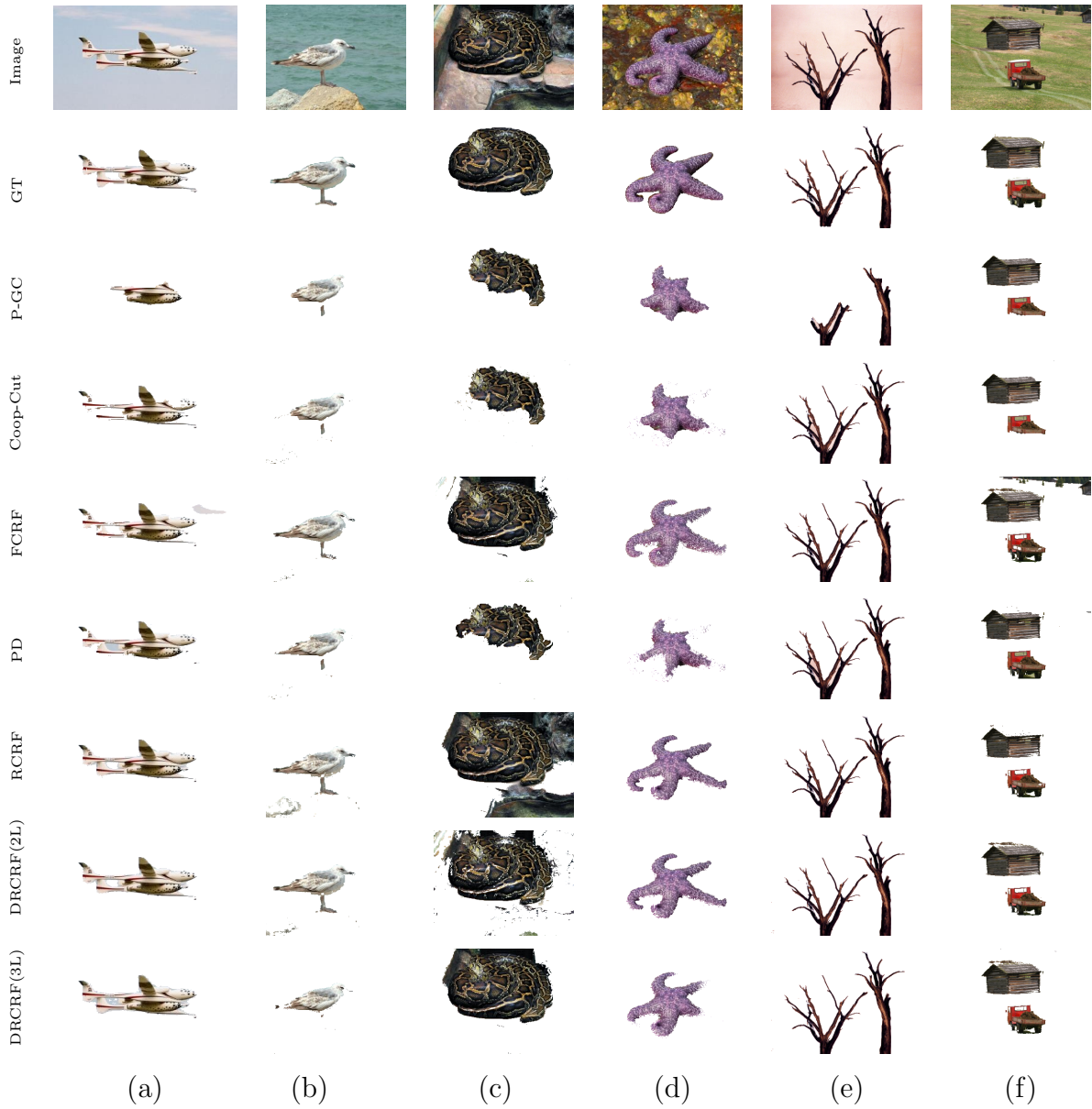
Figure 5.7: Example segmentation results produced by the tested methods on the Weizmann dataset [148] without noise. As seen, the proposed method can preserve elongated boundaries in complex images. Furthermore, the proposed method is capable of dealing with situations characterized by complex and cluttered backgrounds, as is evident in the starfish image (d).
