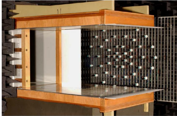
Figure 5.2: KAT setup with lined endplates and microphone array [140].
