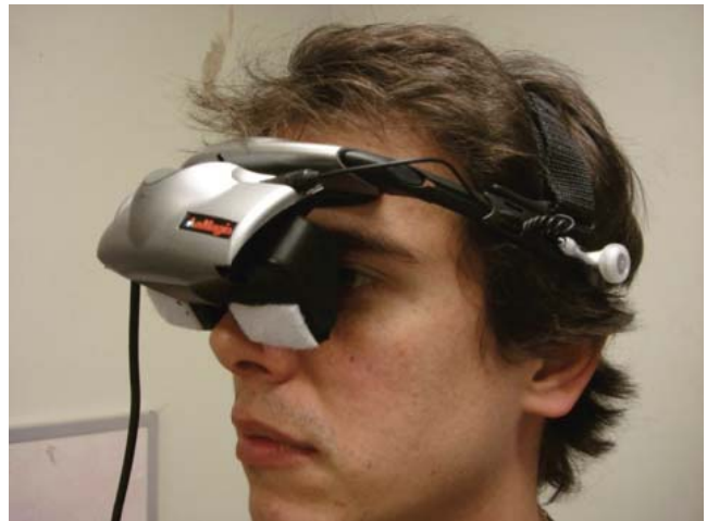
FIGURE 1. The head-mounted goggles used to present dichoptic stimuli for the measurement of suppression and for the restoration of binocular function. Reprinted from Hess RF, Mansouri B, Thompson B. Restoration of binocular vision in amblyopia. Strabismus . 2011;19:110-118.
