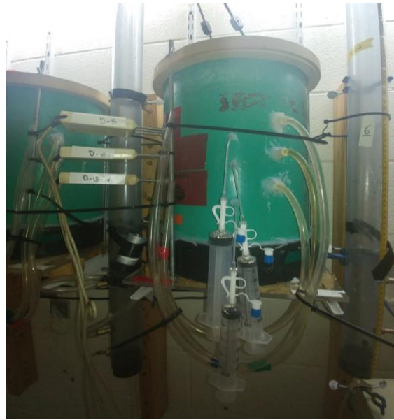
Figure 3-3 One of four cores used in the unsaturated solute breakthrough experiment. The bottom outlet of each core was connected to a Marriot system (far right) that maintained the water table 5 cm above the bottom. Three CS 615 probes (far left) and three tensiometers (right side of core) were installed at 5, 10 and 15 cm bgs to measure SC, water content, and water pressure. Three sampling ports were installed at 7.5, 12.5 and 17.5 cm bgs for biweekly sample extraction.
