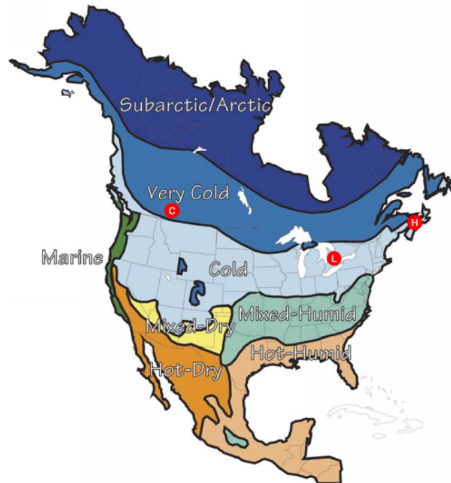
Figure 7.1 North American Hygro-Thermal Regions (Lstiburek, 2011a) C = Calgary, L = London, H = Halifax
