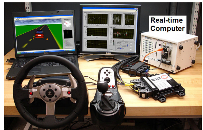
Figure 27. Driving simulator used to further evaluate the performance of the advanced torque vectoring controller (ATVC)
