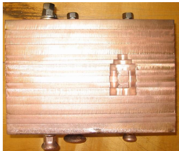
Fig. 8 The laminated tool after brazing process
