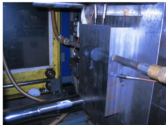
Fig. 11 The laminated injection mould tool during the operation with the sensors installed to investigate the cooling channels performance
