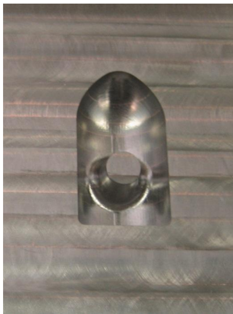
Fig. 10 Inside of the cavity and joined layers
