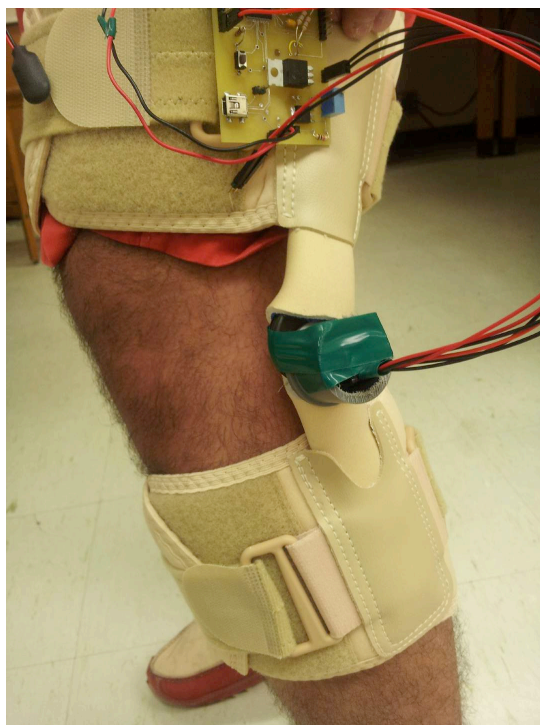
Figure 4.1: Instrumented knee brace used to measure the knee flexion angle in sagittal plane
