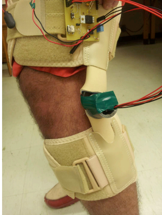
Figure 3.4: Configuration of the sensor system attached to the knee joint
