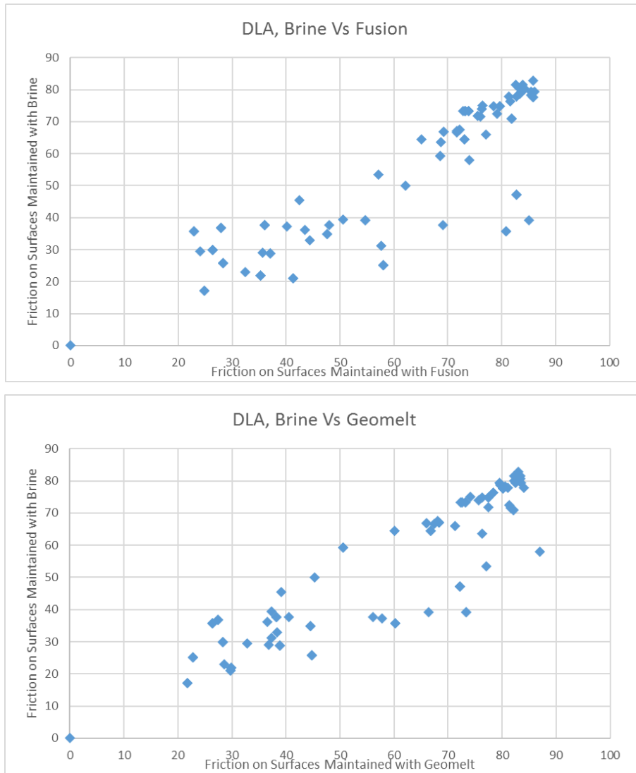
Figure 5.1 Observed Frictions on Sections Treated with Different Materials (DLA Sections)
