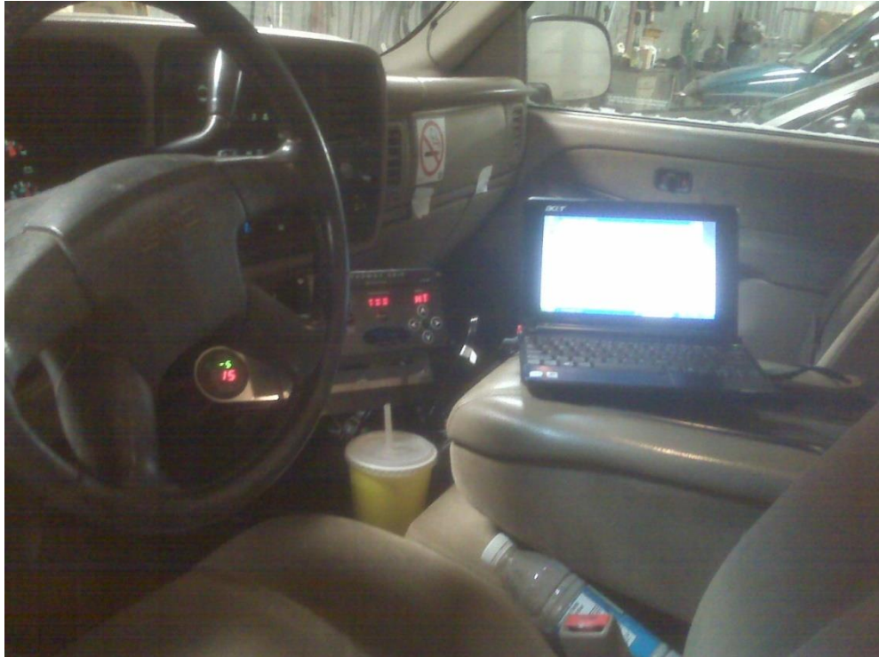
Figure 3.5: Laptop for Data Logging (Laptop with solid state hard drive, purchased specially for the purpose of in vehicle data logging)
