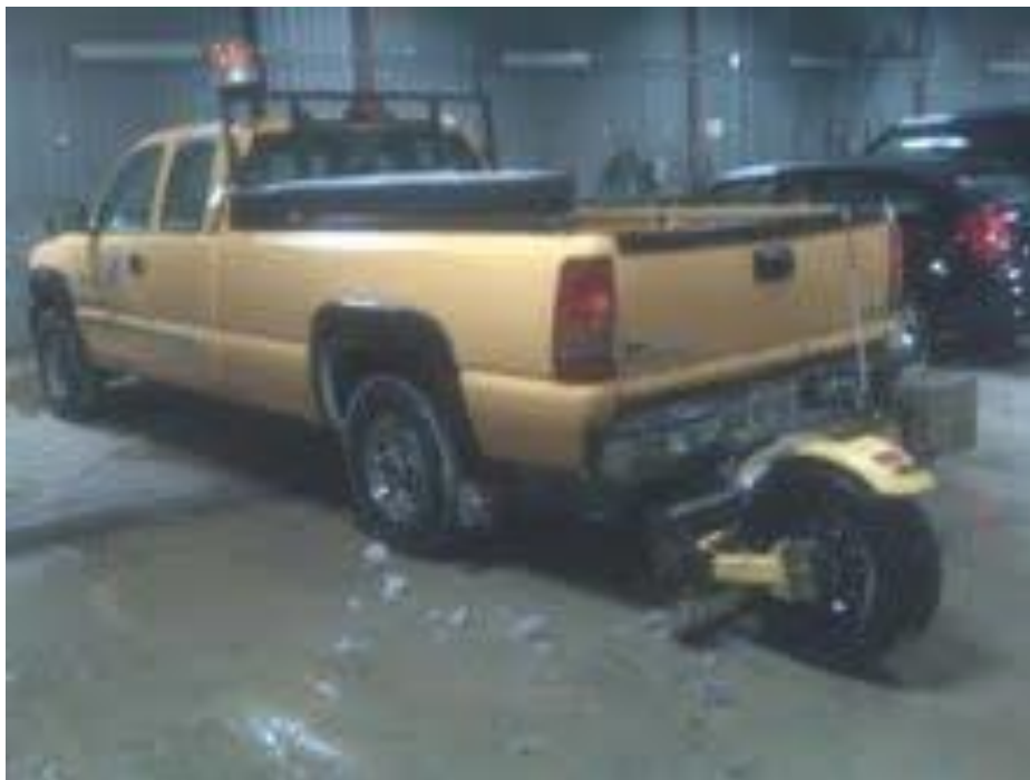
Figure 3.2: Friction Wheel RT3 (Mounted on an S&E Truck)
