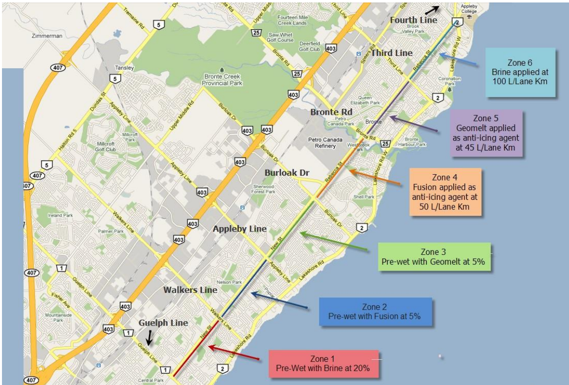
Figure 3.1 Test Site and Zones (Note that New Street ends and Rebecca Street begins at the border of Oakville and Burlington)
