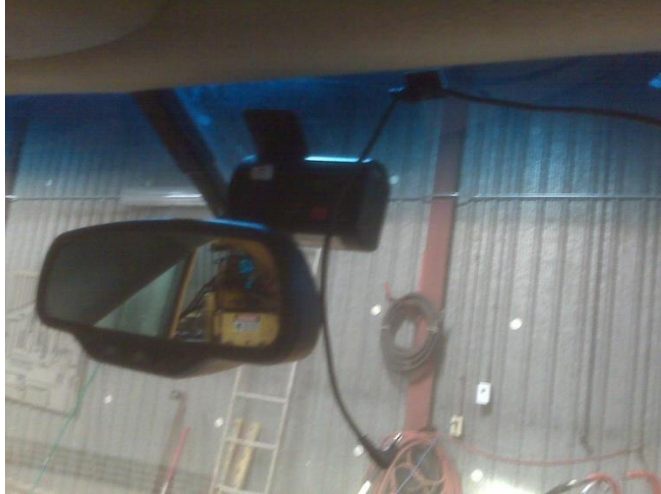
Figure 3.3: GPS and video recorder (Mounted inside an S&E Truck)
