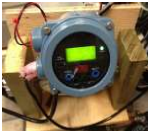
Fig. 5 Refrigerant mass flow meter
