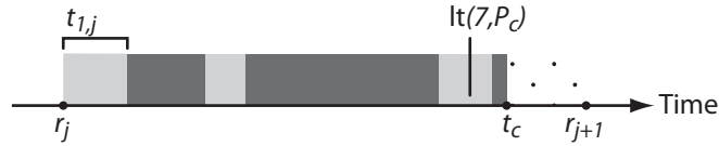
Figure 4.9: An example of a deferral . The shaded blocks indicate the running times of performers 1 . . . 6 whose sum exceeds lt(7, P_c) — the latest P_c -likely start time of performer 7.
