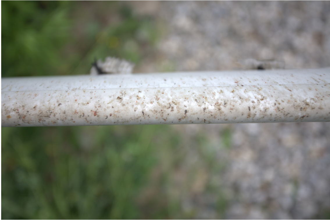
Figure 3.15: Insect fouling on the leading edge of the wind turbine blade
