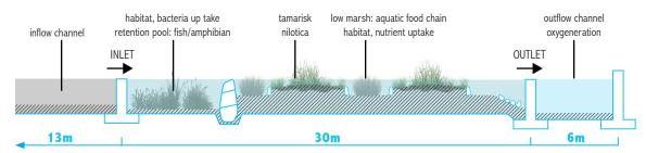
FIG.3.39: Section of a bioremediation cell, reillustrated from the book Out of Water.<sup>48</sup>
