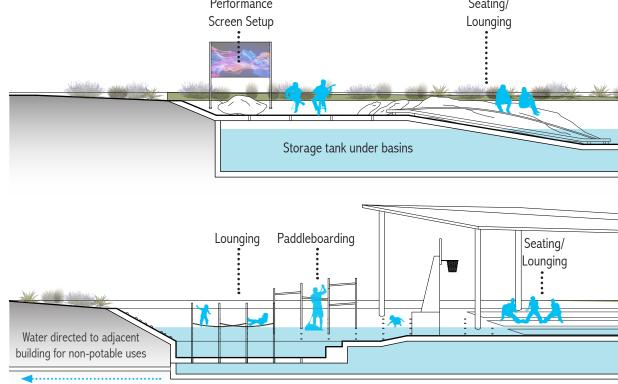
FIG.5.23: Section of retention basins in wet conditions (1:150)
