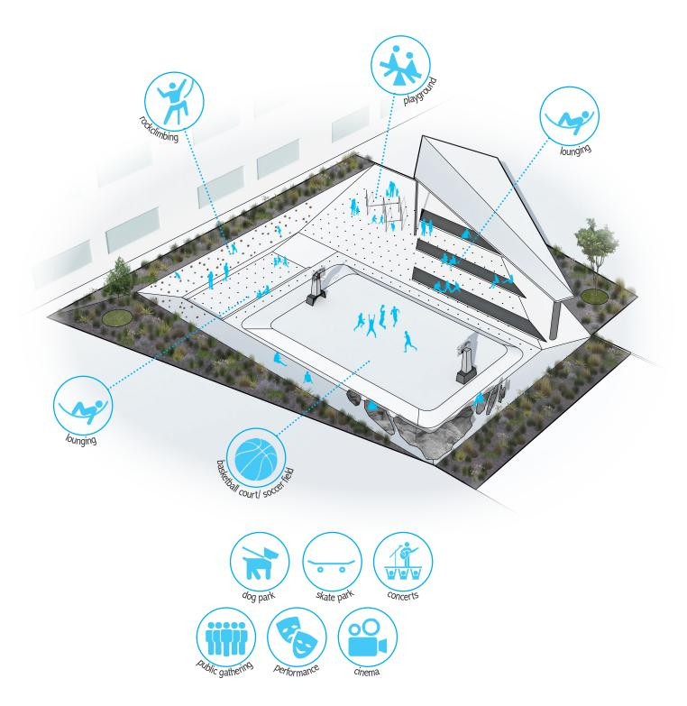
**FIG.5.20:** Type 2 Retention Basin, located in open spaces close to institutional buildings and replacing existing sports ground, such as basketball courts and tennis courts. Bubbles show the types of programs available in the basin during **dry condition.**
