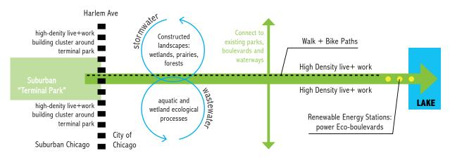
FIG.3.18: Eco-boulevards anatomy, re-illustrated from project drawings.<sup>24</sup>
