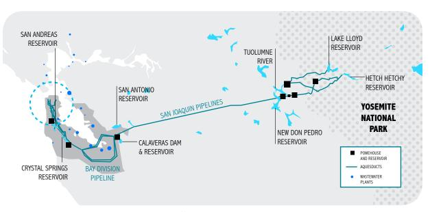
FIG.4.6: Hetch Hetchy Water Delivery system map.<sup>21</sup>
