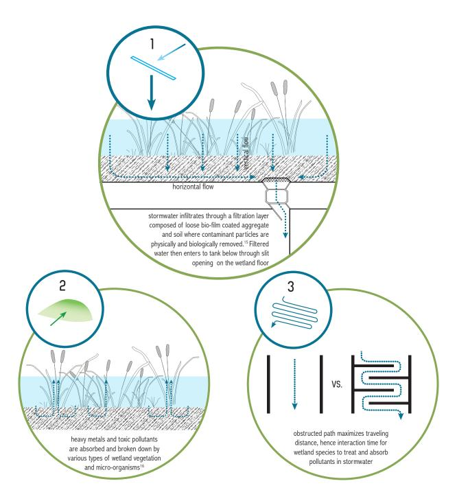
FIG.5.39: Stormwater cleansing processes applied
