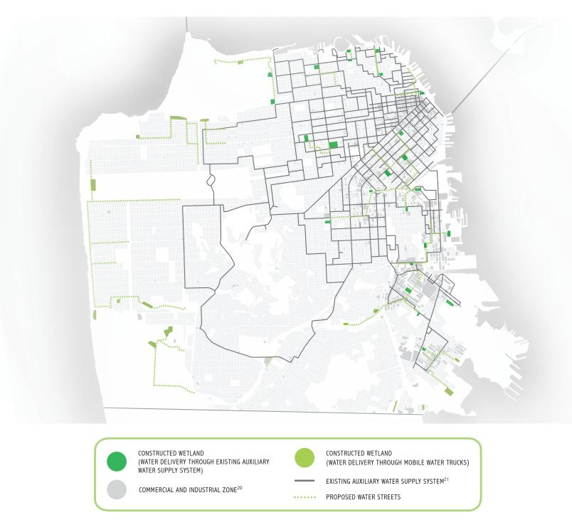
**FIG.5.41:** Constructed wetland water collection and delivery system map (1:80000)
