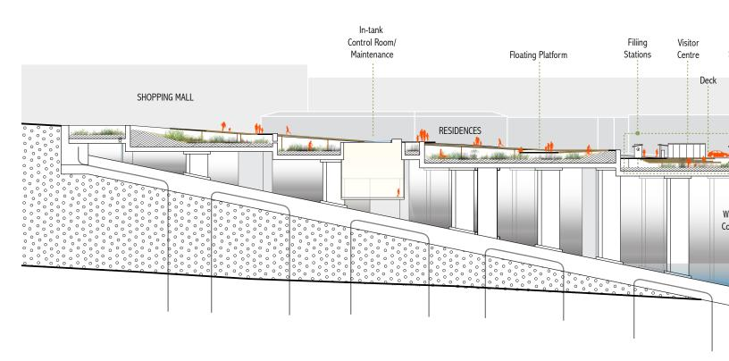
FIG.5.35: Constructed wetland Section B-B (1:700)
