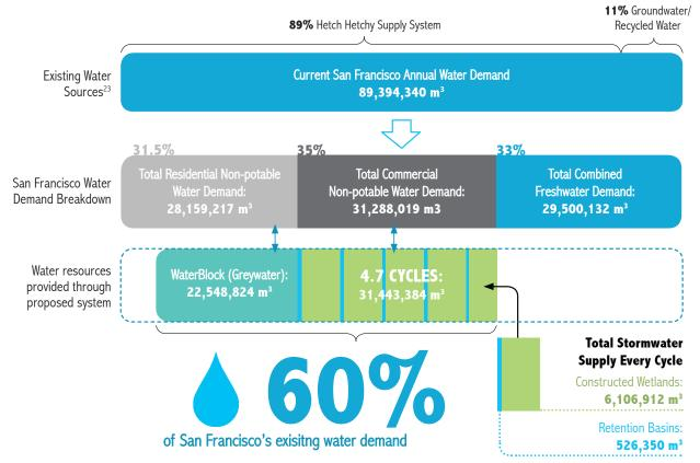
FIG.5.47: Chart showing potential water savings in San Francisco through proposed water system.
