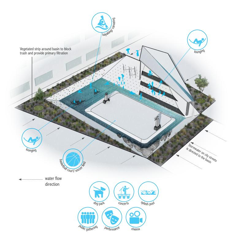
**FIG.5.21:** Type 2 Retention Basin, located in open spaces close to institutional buildings and replacing existing sports ground, such as basketball courts and tennis courts. Bubbles show the types of programs available in the basin during **wet condition.**
