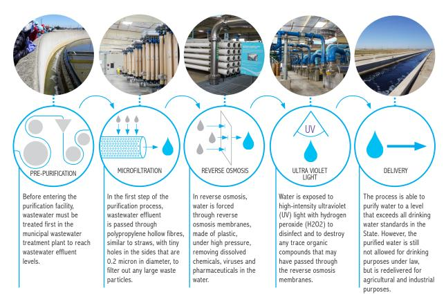
FIG.3.11: Wastewater purification process in the Silicon Valley Advanced Water Purification Facility<sup>19</sup>
