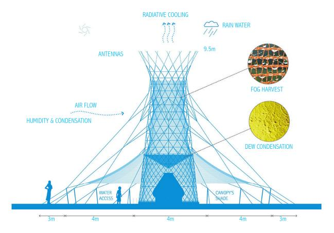
FIG.3.26: Warka Water Tower fog harvesting process
