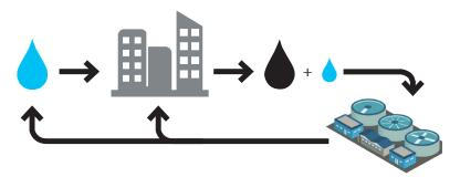
**FIG.3.9:** Close-loop: Water enters system, delivered to end users, but is filtered and treated to be returned for new processes.<sup>10</sup>
