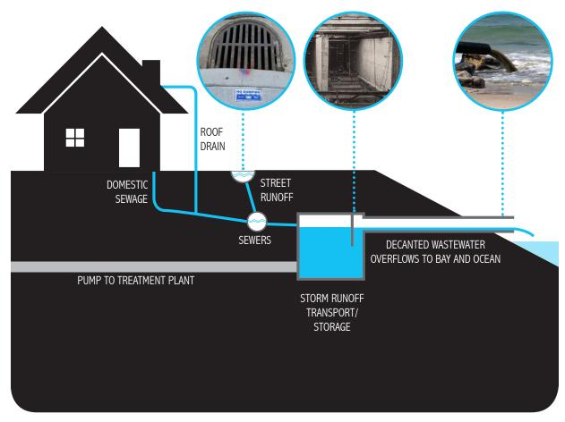
FIG.4.19: San Francisco combined sewer process<sup>36</sup>
