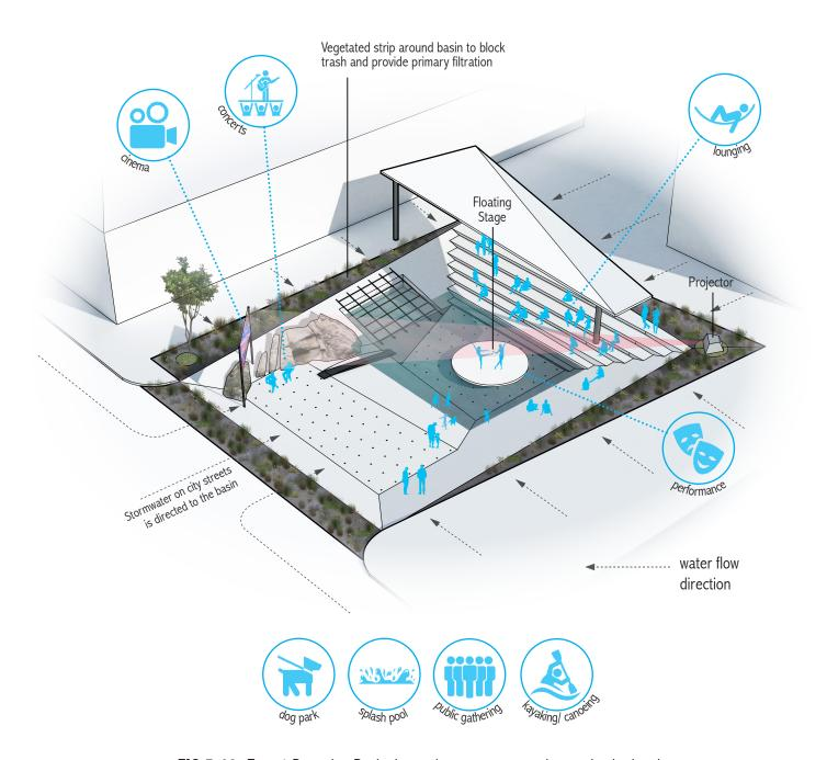
**FIG.5.19:** Type 1 Retention Basin, located at open spaces close to institutional buildings. Bubbles show the types of programs available in the basin during **wet condition.**
