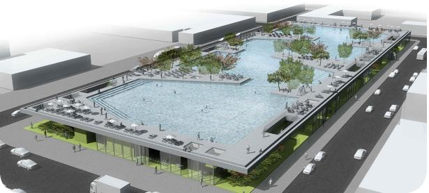
**FIG.3.22:** A render of the roof after a storm event, rainwater fills the sunken areas and forms pools for the community.
