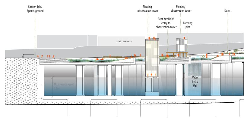
FIG.5.34: Constructed wetland Section A-A (1:700)
