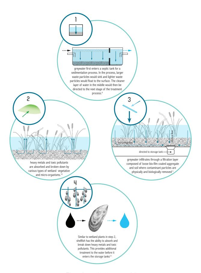
FIG.5.15: Greywater cleansing processes applied
