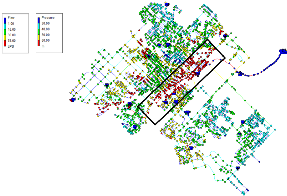
Figure 6.15: Model output of pressure monitoring junctions. The high-pressure belt is delimited with a black rectangle.
